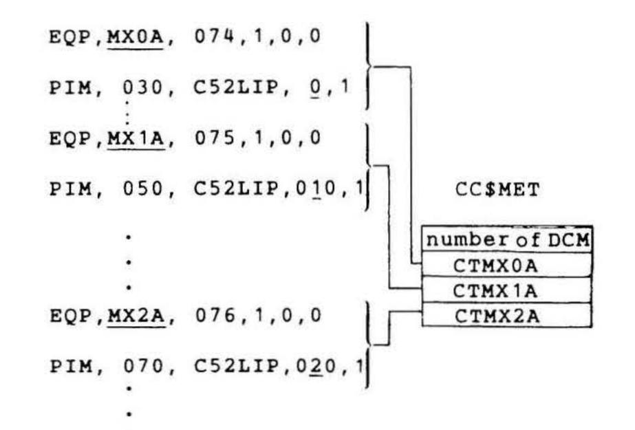
For each EQP card defining a DCM six PIM directives are needed to define the six DCM interrupts.
