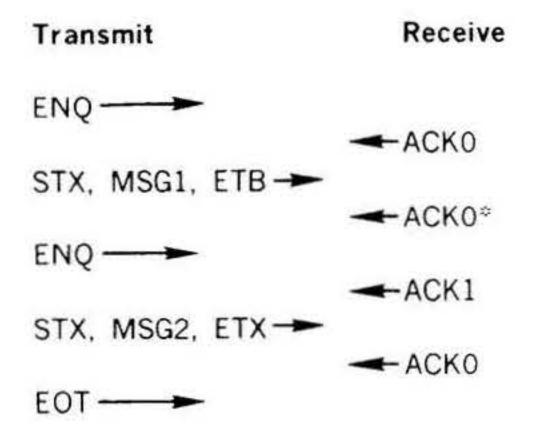
\* ACK1 Character changed to ACK0 due to line failure.
