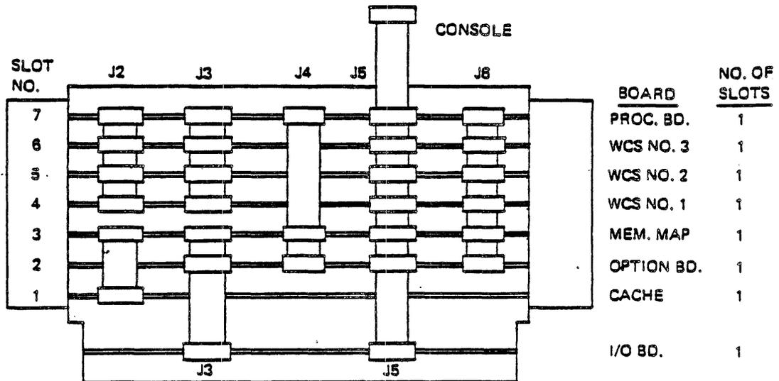
Figure 2-2. 70 Configuration with Three WCS II Boards
