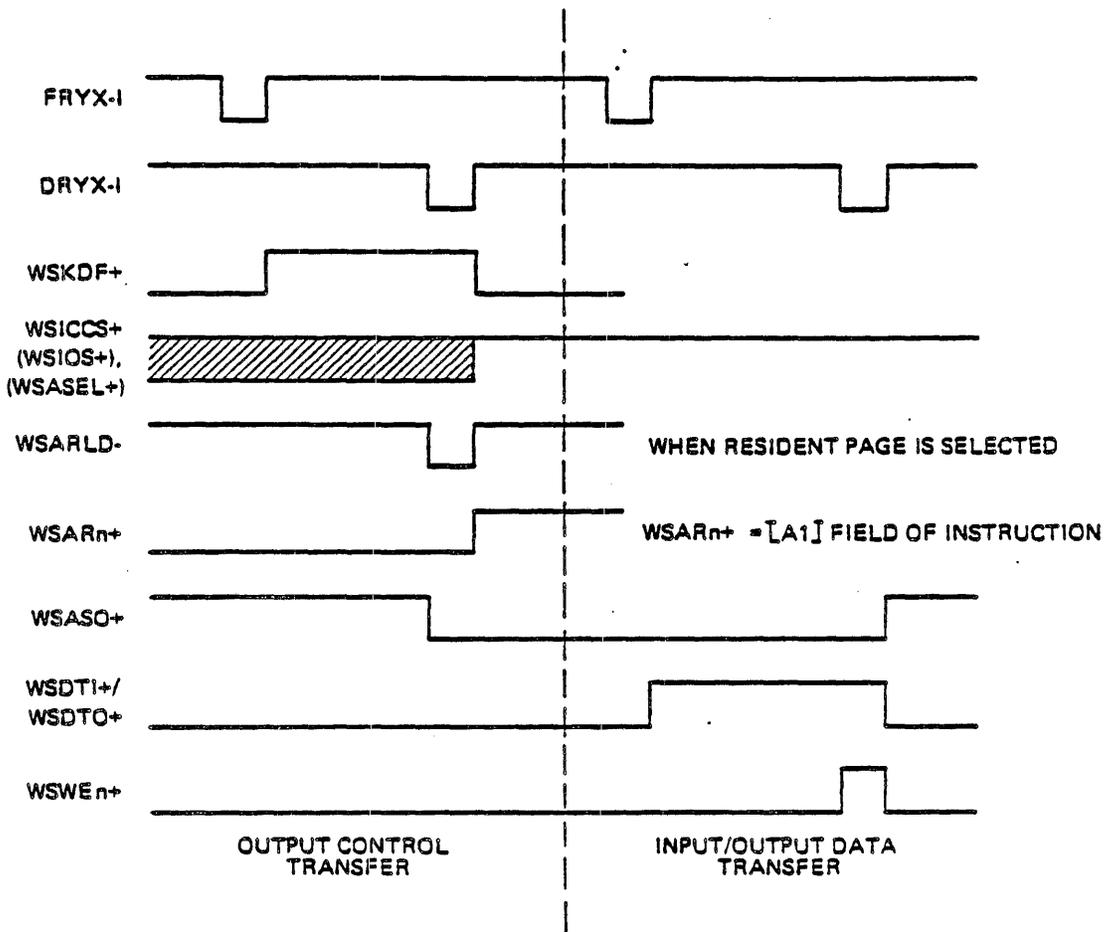
Figure 4-11. Programmed Input/Output Transfer to the Selected Control Store
