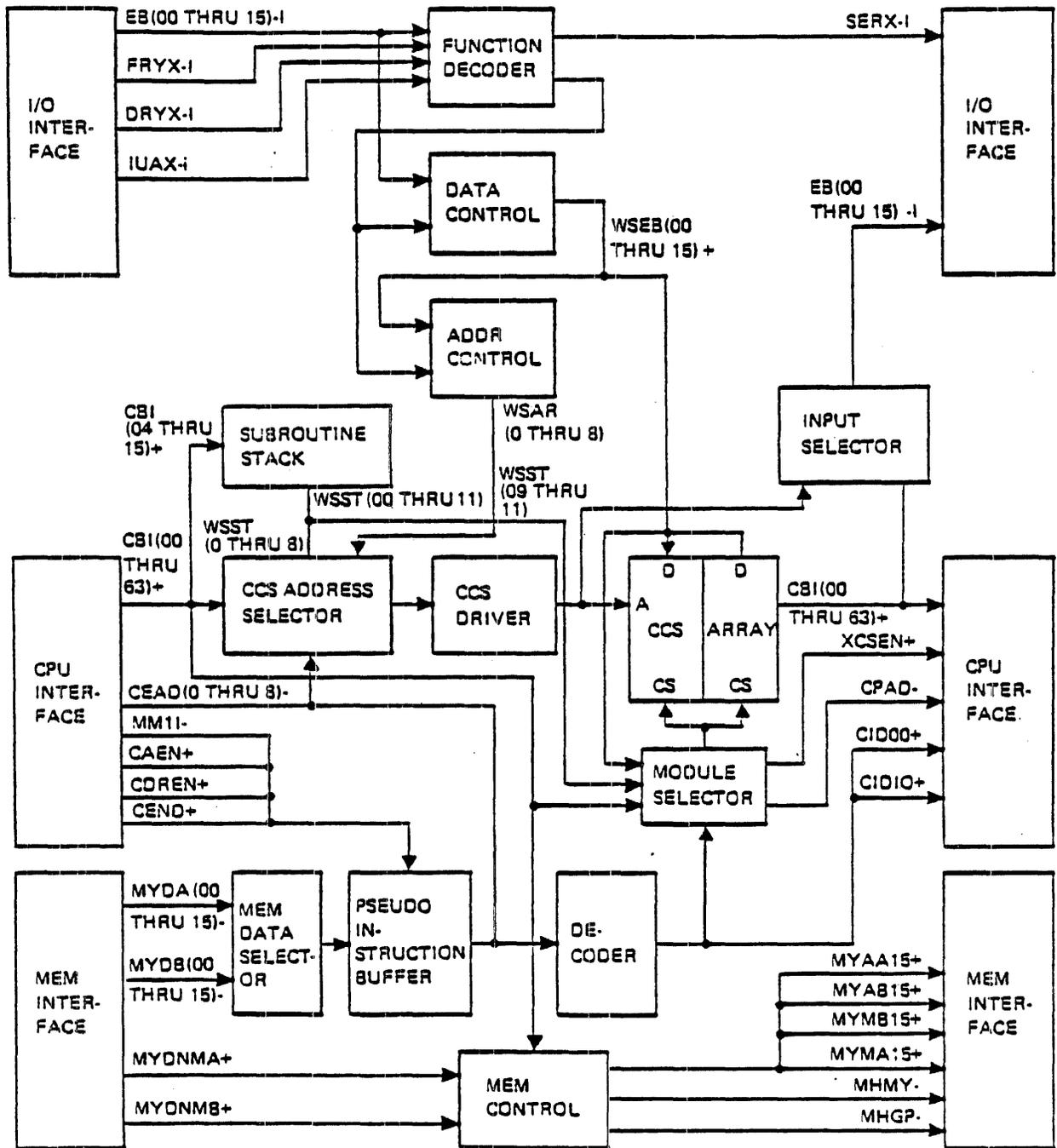
Figure 4-1. WCS II Functional Block Diagram
