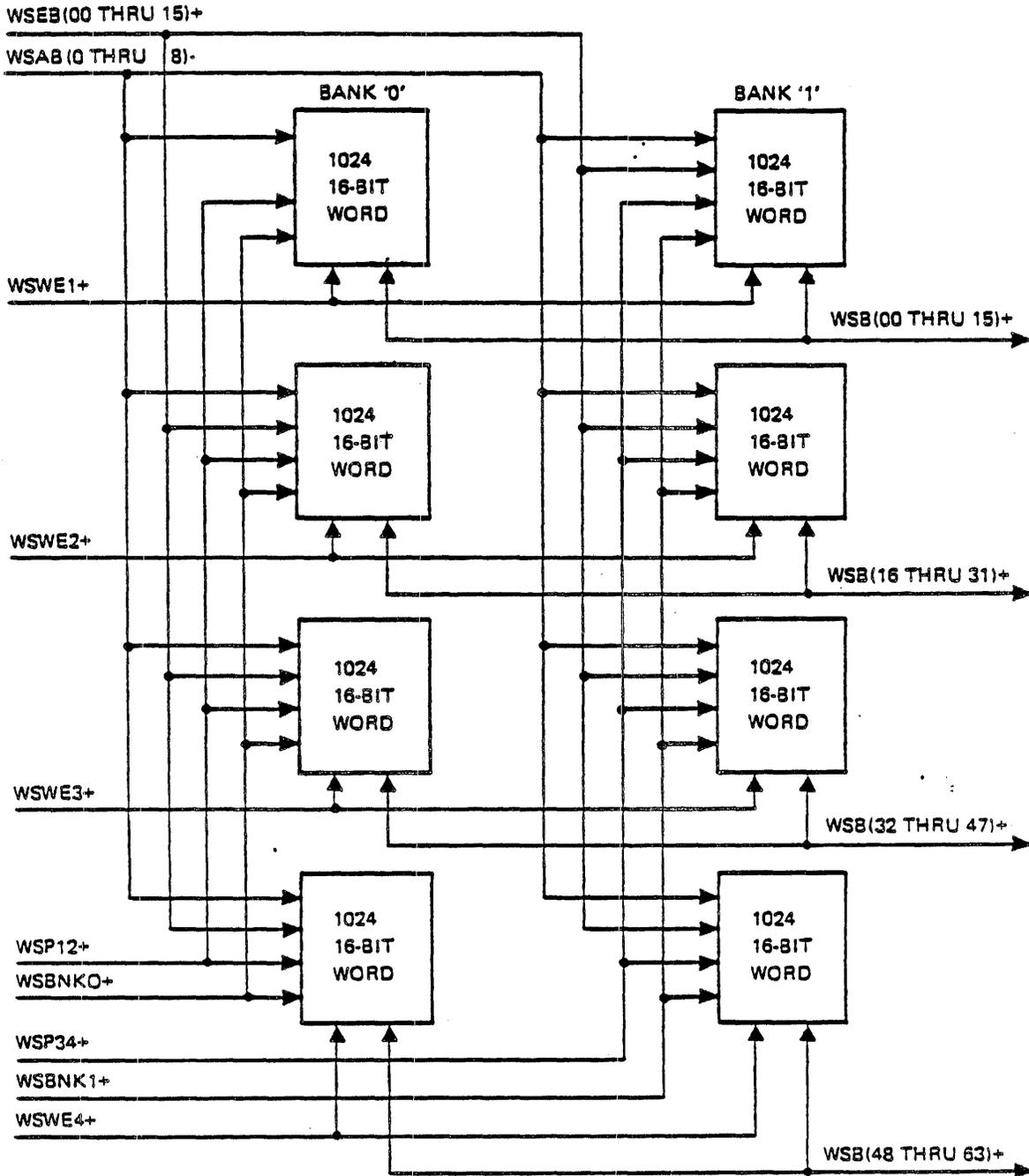
Figure 4-3. CCS Array Block Diagram
