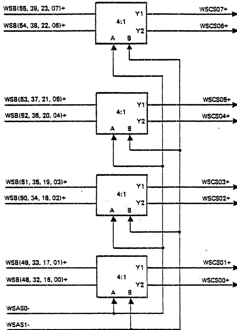
Figure 4-6. Four-to-One Data Multiplexor
