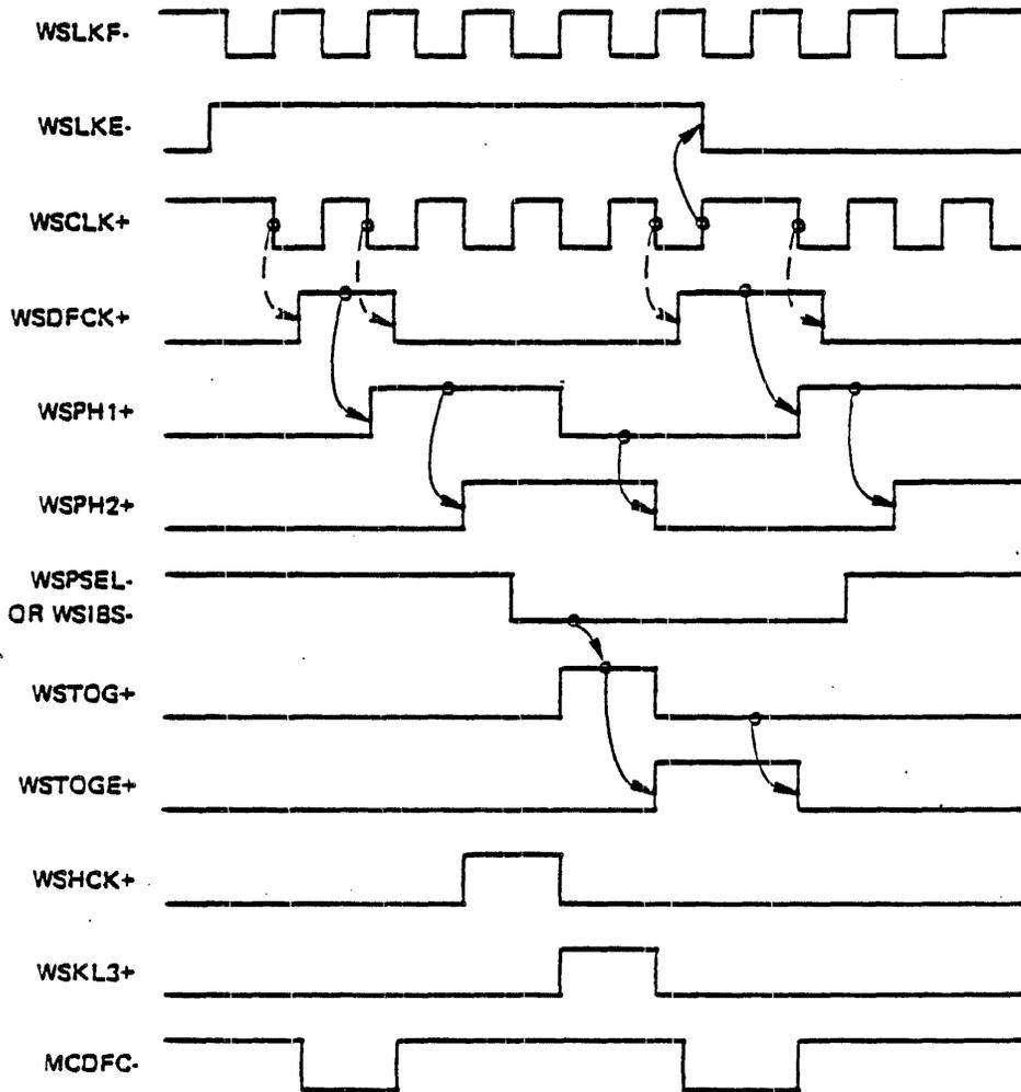
Figure 4-10. WCS II Clock Control (when WCS II is Selected via WSPSEL- or WSIBS-)
