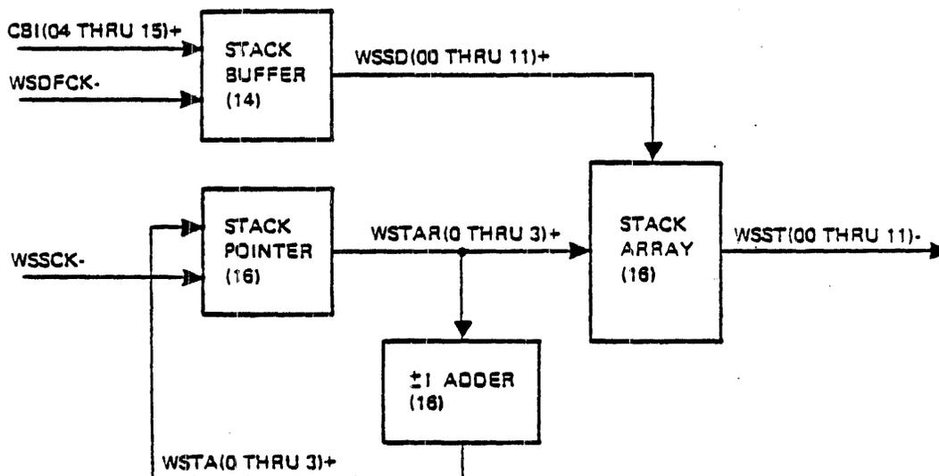
Figure 4-7. Subroutine Stack Block Diagram
