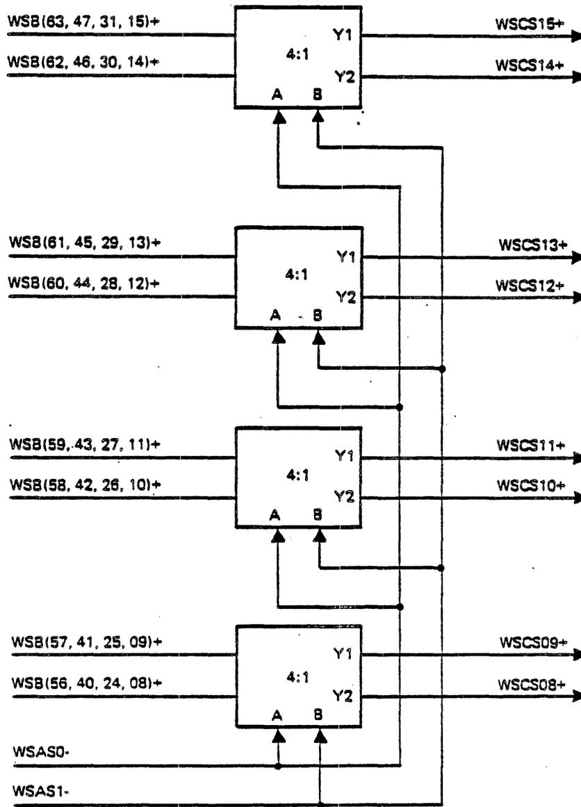
Figure 4-6. Four-to-One Data Multiplexor
