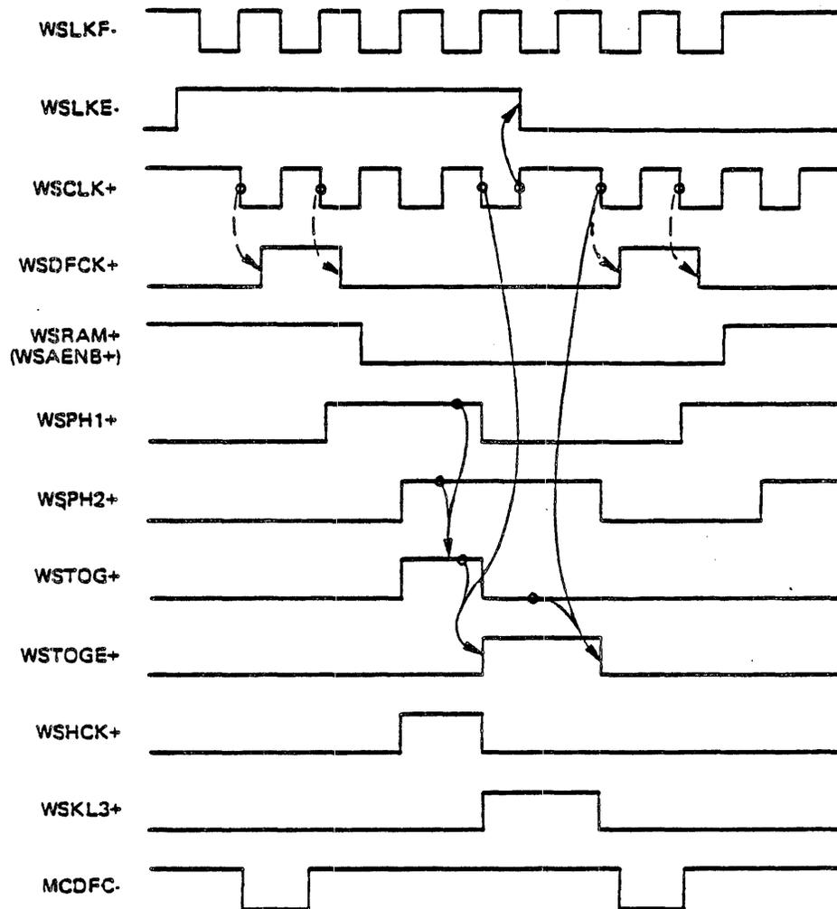
Figure 4-9. WCS II Clock Control (when WCS II is Selected via WSRAM+ or WSAENB+)
