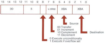
The X, B, and A Register contents can be logical "ORed," cleared, transferred, set to a common value, complemented, "NORed," incremented, decremented, and, if desired, executed conditionally on an overflow. Sequences of micro-commands can be used to perform additional logical functions customary in a system environment.
