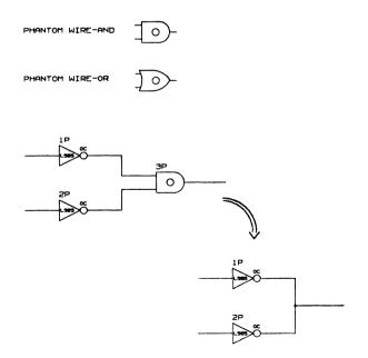
Figure 4-1. Wire-OR and Wire-AND Phantom Bodies
