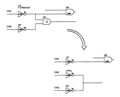
Figure 8-5. Replacing Phantom Bodies with Wire-Ties
