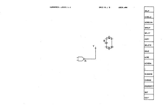
Figure 42. Starting a wire fixed in the horizontal direction
