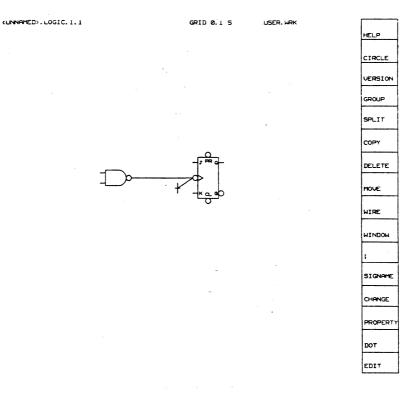
Figure 12. Wire connected to a second pin
