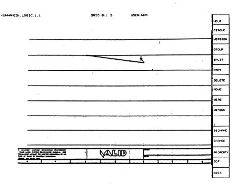
Figure 30. Wire snapped to nearest grid intersection
