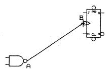
To create an orthogonal wire, start the wire at point A by pressing the yellow button.
