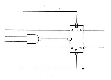
Figure 14. Wires connected to a pin at one end only
