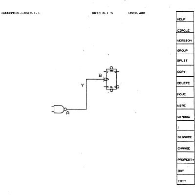
Figure 47. Redirect the wire with the white button and place the wire down with the blue button. When ending a wire that does not terminate on a pin, the use of the blue button makes it convenient to generate the zero-length segment required to terminate a wire; the cursor need only be moved close to the ending vertex and the blue button pressed.
