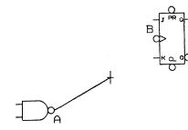
To complete the wire, press the white or green button again, then press the yellow button to bend the wire at Y. Drag the wire towards the clock input and press the blue button twice to snap to the connection and lay the wire down.
