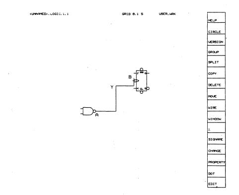
Figure 46. To finish the connection, move the cursor to point B
