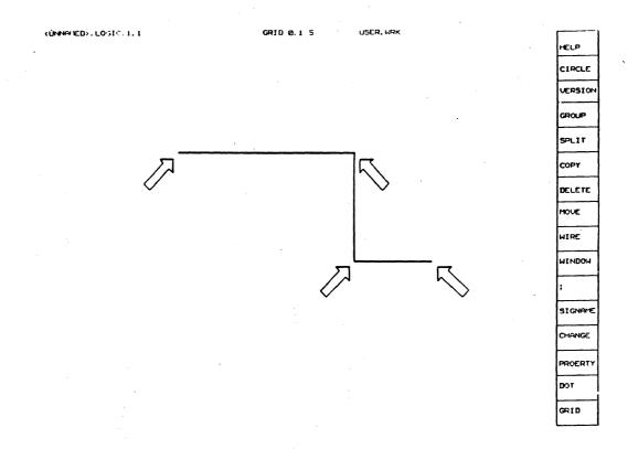
Figure 32. Wire -- vertices at each end and corner
