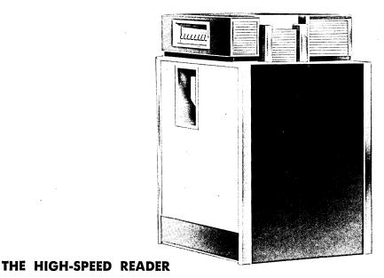
The High-Speed Reader is a major input component of the UNIVAC Solid-State 90 Magnetic Tape System. It reads data into the system from punched cards at a speed of 450 cards per minute.
