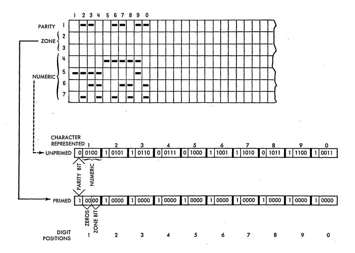
FIGURE 8. Numeric Representation on Tape and in the Computer in UNIVAC XS-3 Code
