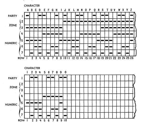
FIGURE 7. Numeric and Alphabetic Representation on Tape (with Parity Bits)
