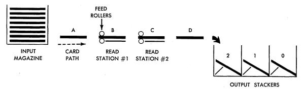
FIGURE 1. Functional Diagram of the Transport Mechanism of the High-Speed Reader
