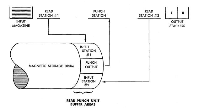
FIGURE 16. Relationship of Punch, Read Stations to Buffer
