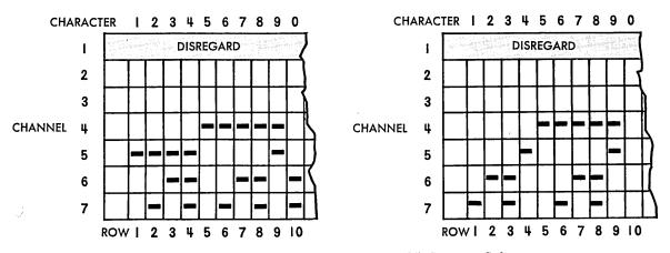
FIGURE 5. Numeric Representation on Tape in UNIVAC XS-3 Code and in Computer Code
