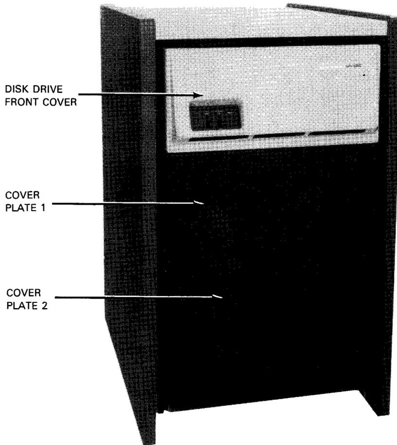
*Figure 2—2. Disk Drive Cabinet with Single Drive*
