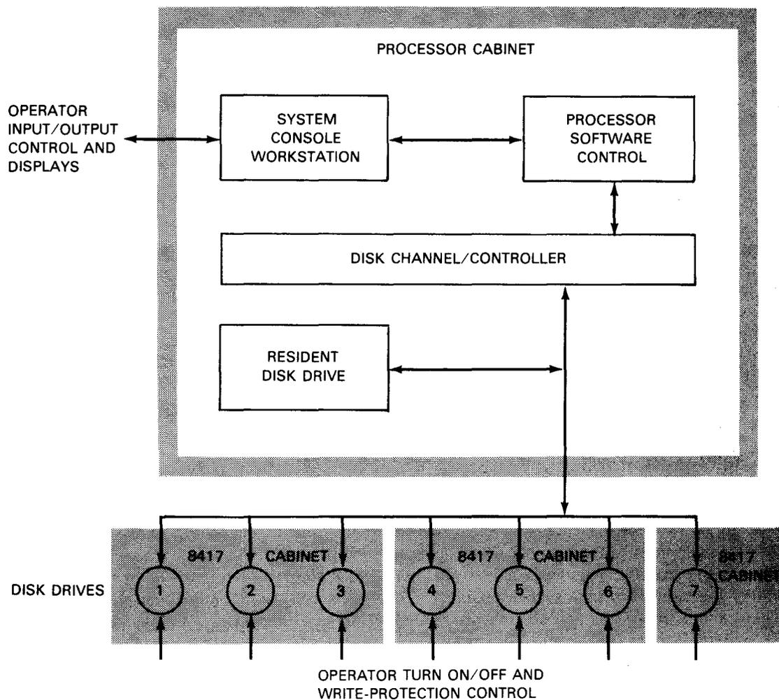
Figure 2-1. 8417 Disk Subsystem Control Directions
