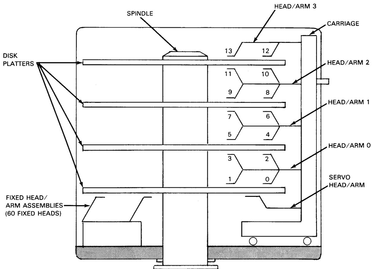
Figure 2-3. Disk Drive Head Disk Assembly
