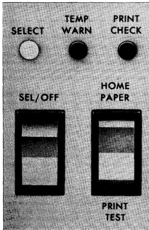
Figure 4-6. Console Printer Operator Panel
