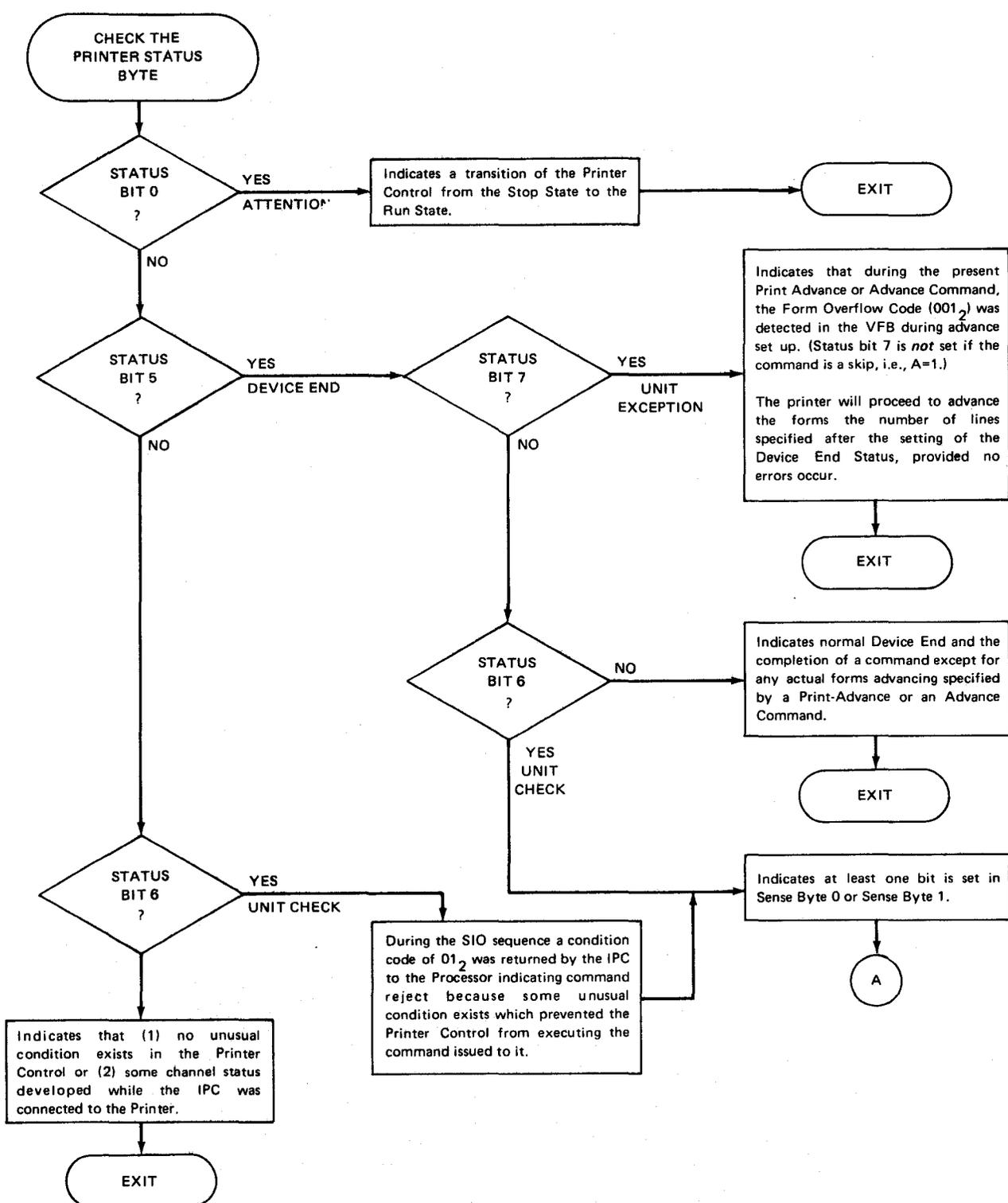
Figure 7-15. Conditions Indicated by Status Byte
