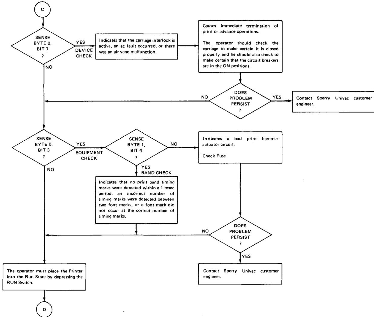
Figure 7-17. Equipment Check Error Recovery Flowchart (Part 2 of 2)
