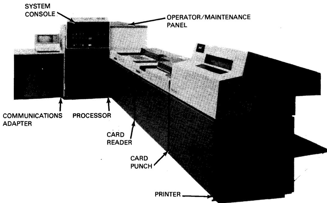
Figure 1—1. 90/30 System With Integrated Peripheral Devices
