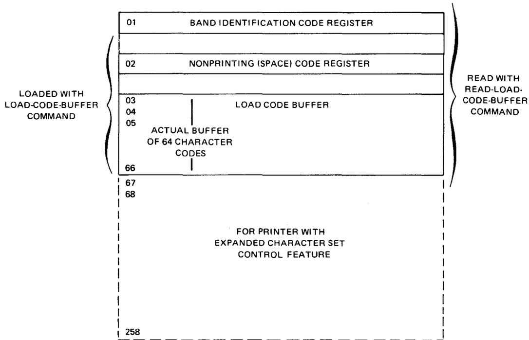
Figure 7—6. Load Code Buffer Array
