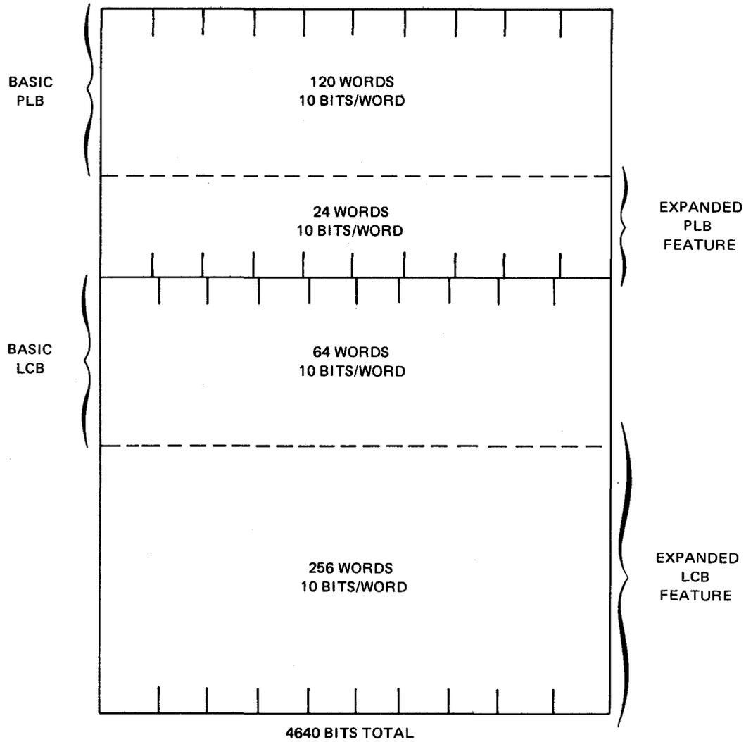
Figure 7-7. Print Line Buffer and Load Code Buffer Map
