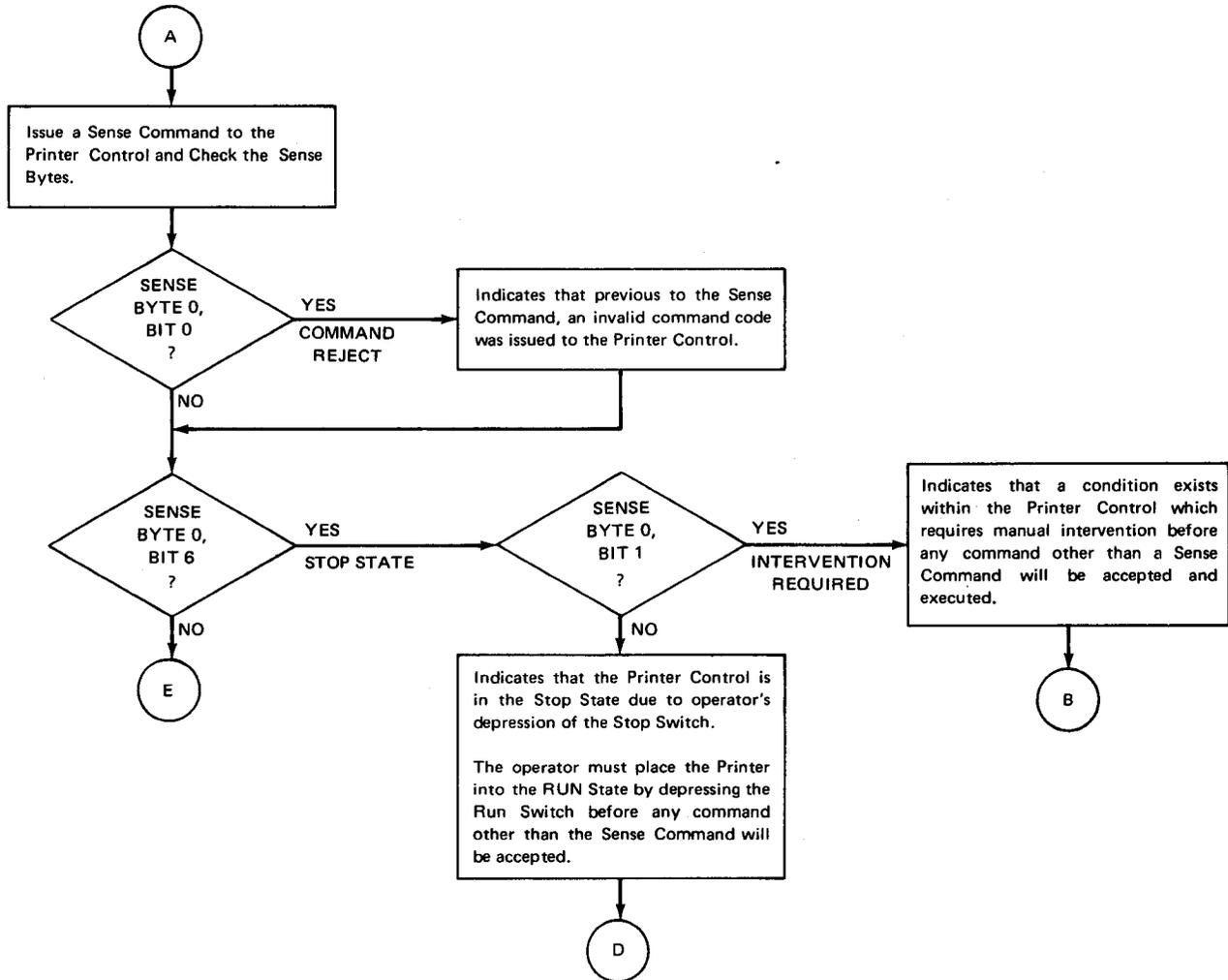
Figure 7-16. Intervention Required Error Recovery Flowchart
