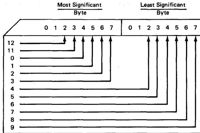
Figure 5-5. Image Mode Byte Formats on Card
