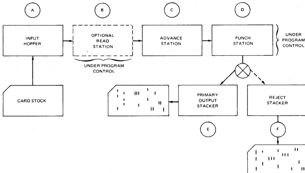
Figure 6—3. Card Punch, Block Diagram
