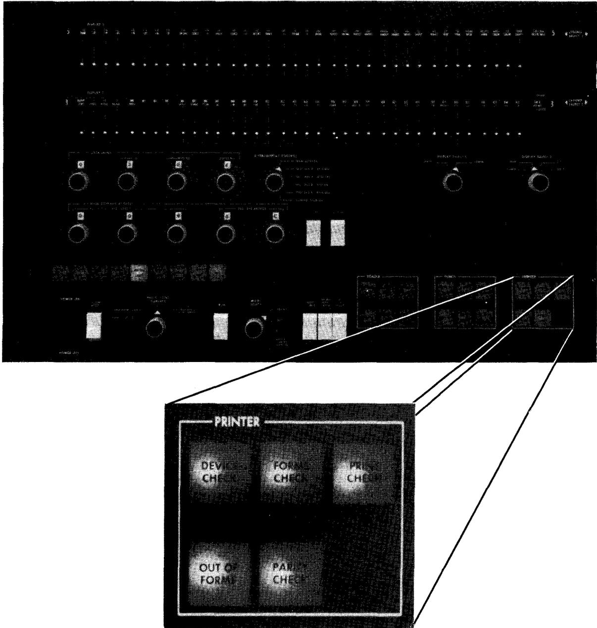
Figure 7-13. Processor Operator/Maintenance Panel Showing Printer Error/Fault Indicators
