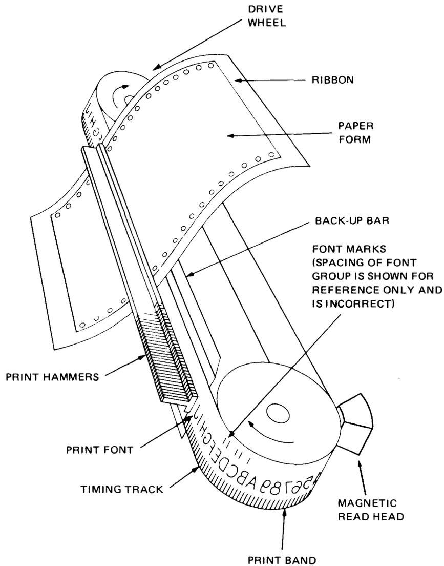
Figure 7-11. Print Function, Schematic Diagram
