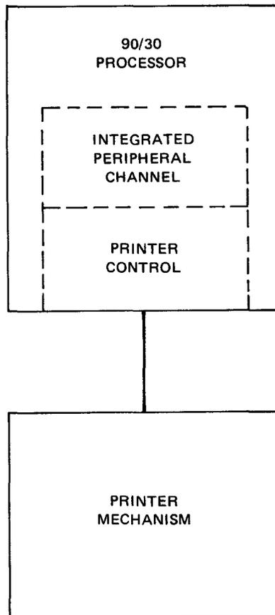
Figure 7—2. Printer Functional Arrangement
