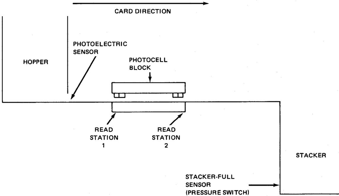
Figure 5-4. Card Path Through Card Reader
