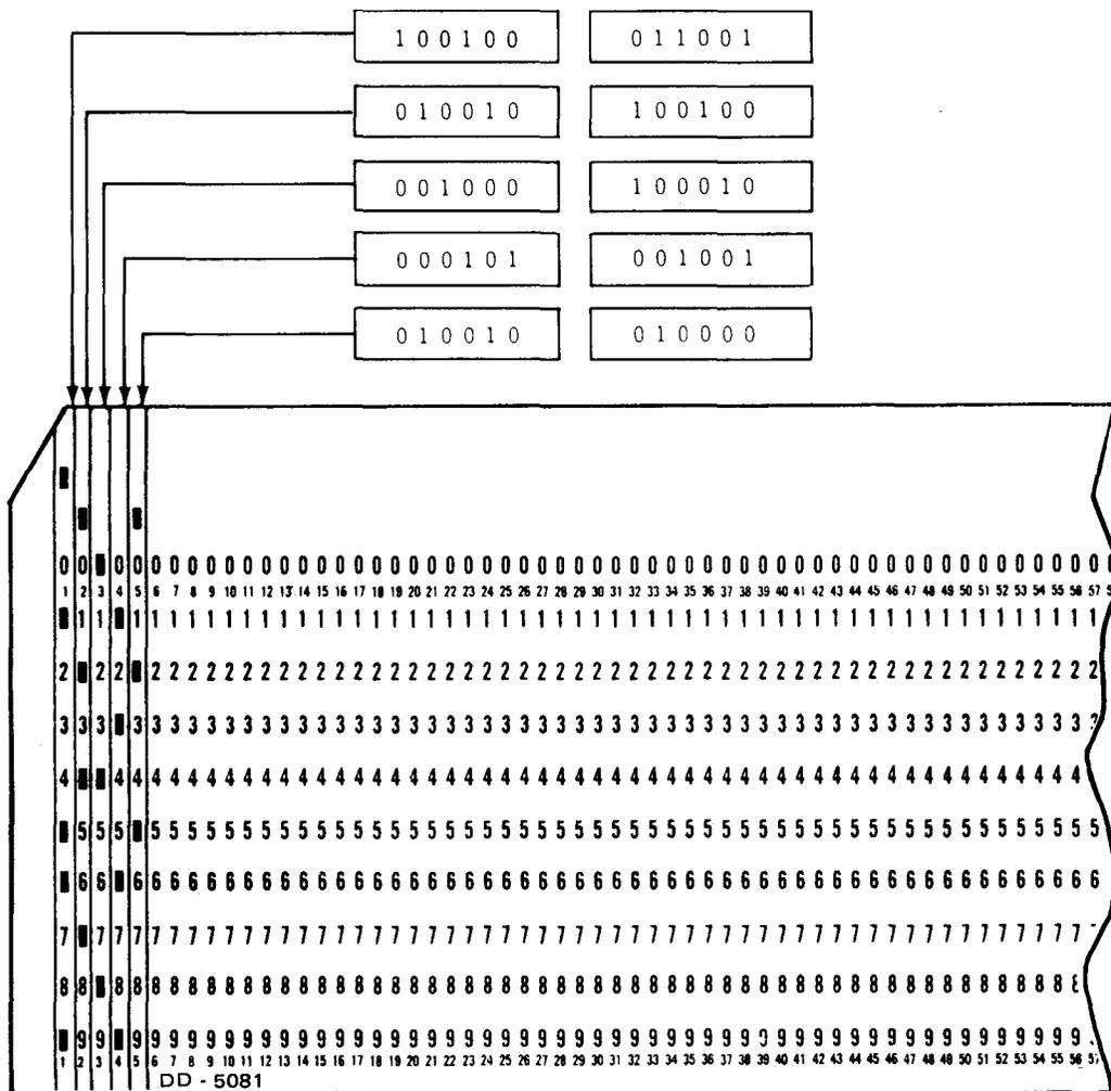
Figure 6-6. Relationship of Data Bytes to Card Punches (Image Mode)
