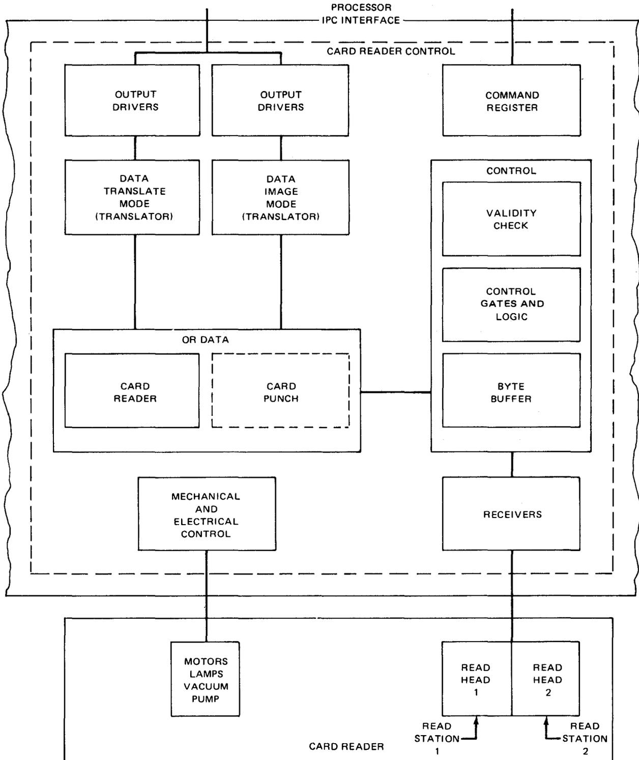
Figure 5-3. Card Reader Control, Block Diagram
