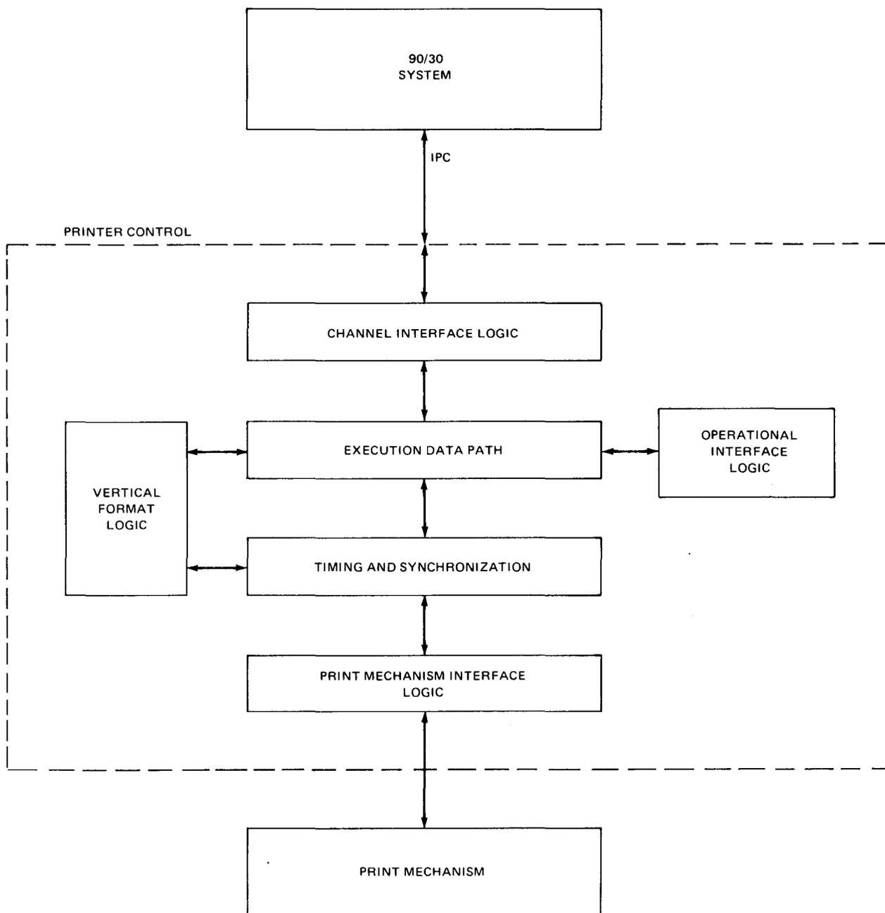
Figure 7-4. Printer Control Circuitry
