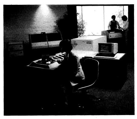
The Sperry System 80 is Sperry's general-purpose mid range system. The Models 4 and 6, shown here, provide up to 4MB of main memory and up to 1.3GB of disk storage; the Model 6 features High Performance Control Storage (HPCOS) for increased central processor speed. The top of the line Model 8 can support up to 8MB of main memory and 12GB of disk storage.
