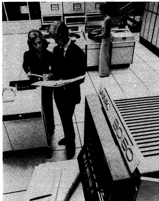
The UNIVAC 90/60, as a result of performance enhancements and price cuts announced in August 1976, now reportedly surpasses the IBM 370/138 in performance and nearly matches it in price. The 90/60 can have from 524K to 2 million bytes of MOS memory with a cycle time of 600 nanoseconds per 4-byte access.
