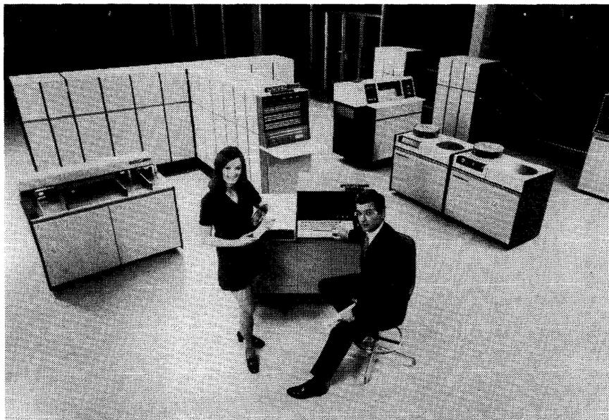
This view of a fairly small, disc-oriented UNIVAC 90/70 configuration shows the CRT-equipped System Console in the foreground and the Central Processor at left rear.
