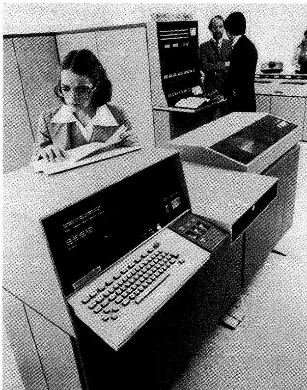
*The UNIVAC 90/80, the newest and largest current member of the Series 90 family, offers from 524K to 4 million bytes of MOS main memory with a cycle time of 450 nanoseconds per 8-byte access. Instruction processing and I/O processing functions are segregated into two separate processors for increased efficiency.*
