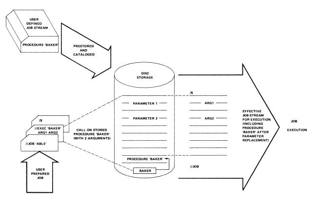
Figure 6–6. Information Flow – OS/7 Cataloged Job Control Procedures
