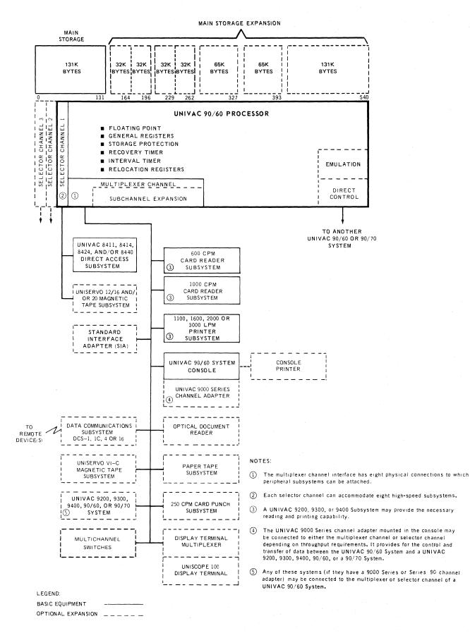
Figure 2–2. UNIVAC 90/60 System Hardware
