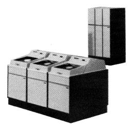
UNIVAC 8411/8414 Disc Subsystem
