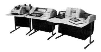
The UNIVAC DCT 1000 Data Communications Terminal is a fully buffered 30-characrer-per-second incremental printer which can be expanded to include a keyboard, card reader, card punch, paper tape reader/punch, and an auxiliary printer. The DCT 1000 transmits or receives data from a local or remote processor or to a remote DCT 1000 in a conversational or batch mode.
