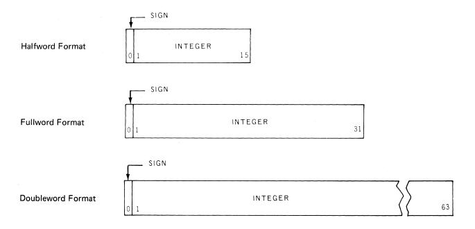
When held in one of the 16 general registers, a fixed-point number is generally treated as a 32-bit operand. When a halfword fixed-point number is called from storage and loaded into a register, the sign is extended to the left to fill the fullword register. The contents of the register are then handled as a fullword operand in fixed-point arithmetic operations.
