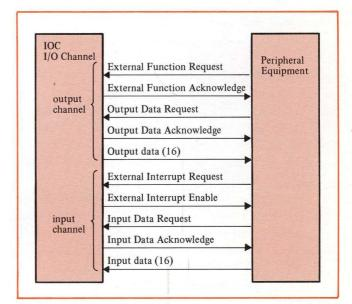
Figure 5. IOC Channel Interface
