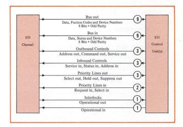
Figure 4. Processor/Peripheral Channel Interface
