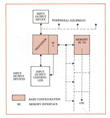
Figure 2. Basic and IOC Configuration
