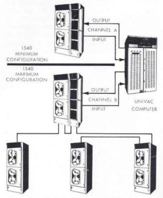
Figure 2. UNIVAC 1540 Magnetic Tape Units and Computer Configuration
