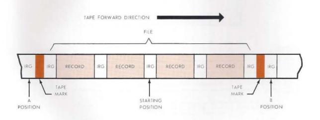
Figure 11. Magnetic Tape Unit – Tape File
