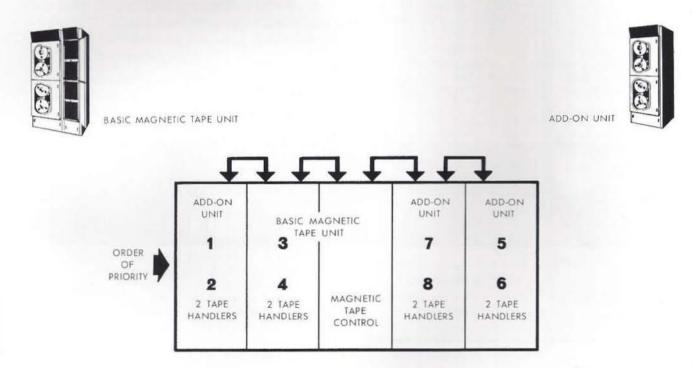
Figure 5. Type 1540 Magnetic Tape System (Maximum Configuration)
