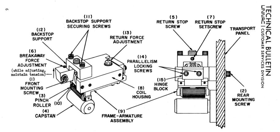
Figure 1. Solenoid Adjustments
