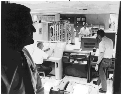
The ARTS I system in Atlanta, the SPAN system in Indianapolis, and the NYCBAN system in New York used the UNIVAC 1218 computers. The ARTS IA system at the New York CIFFR used the UNIVAC 1219B computers (pictured right). Operational software ran in two 1219B computers; one provided Track Processing (TP) functionality and the second one provided Display Processing (DP) functionality. The executive program was a short, endless loop that called all the major program functions (e.g., Tracking).
