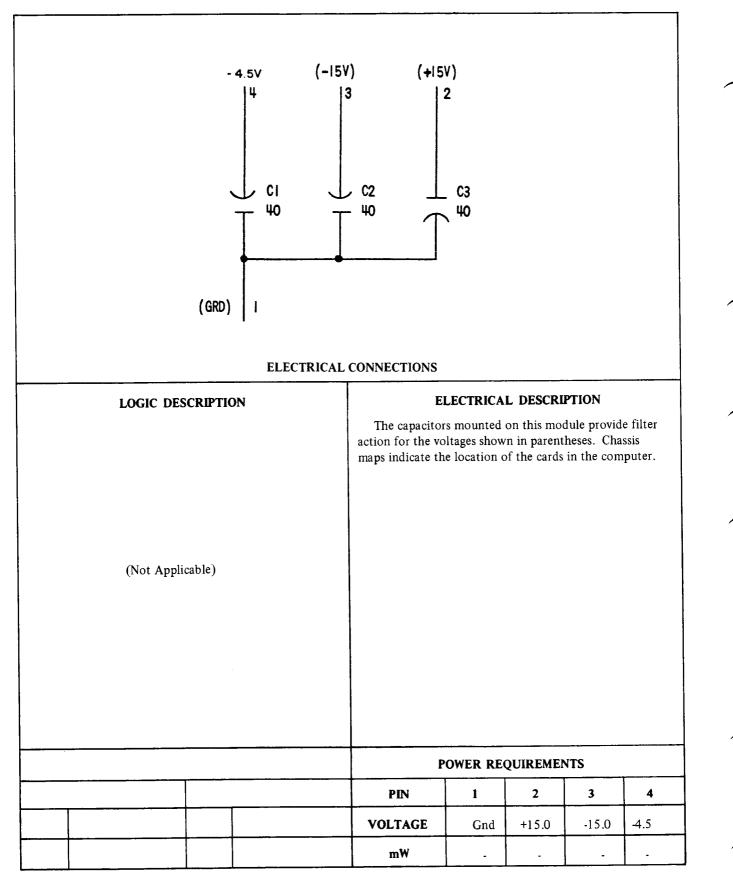
Figure 7-41. Capacity Assembly - #3, Card Type 7003180
