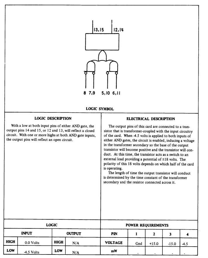
Figure 7-56. Driver-Digit Amplifier, Card Type 7003780
