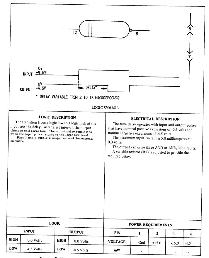
Figure 7-42. Time Delay - 2 to 15 usec, Card Type 7003480
