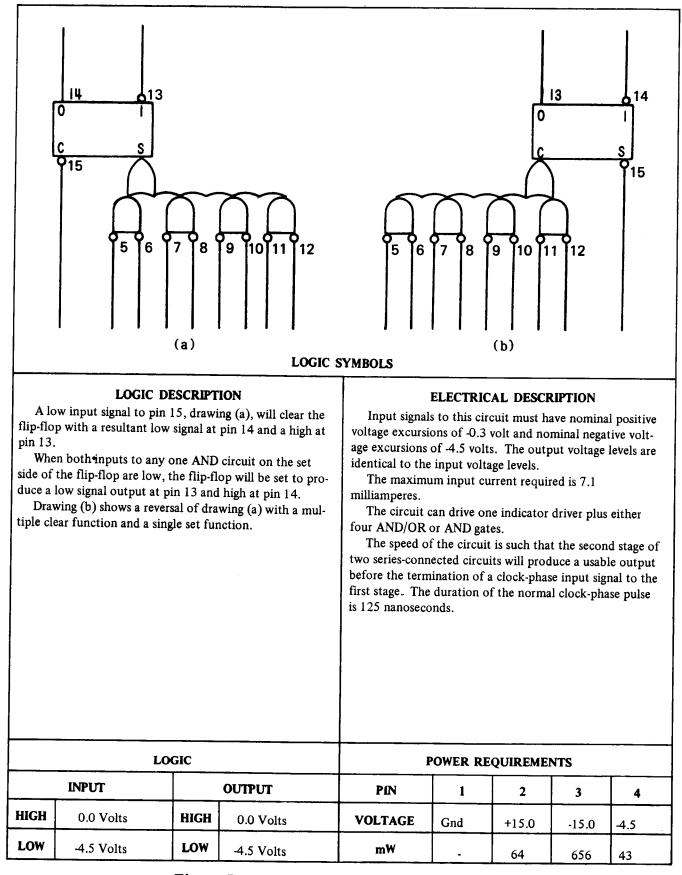
Figure 7-16. Flip-Flop, Card Type 7002000
