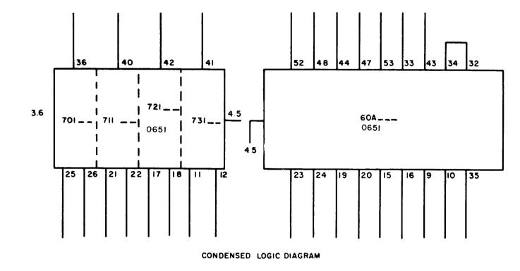
Figure 7-78. Logic Symbol of Sense and Inhibit Amplifier on 7500651 Module
