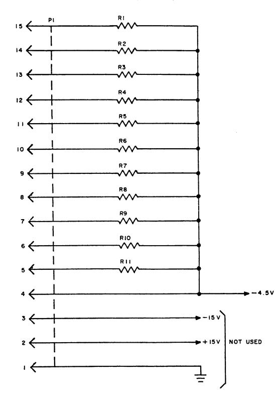
Figure 7-59. Resistor Assembly, Module 7109000 Schematic Diagram
