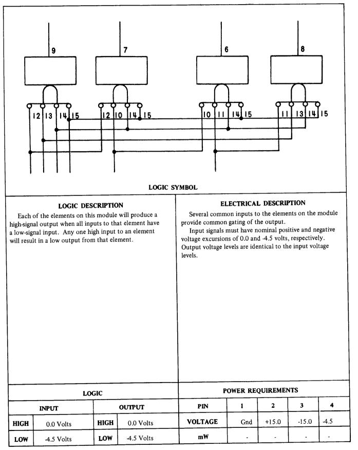
Figure 7-49. Transformer Driver, Card Type 7003680
