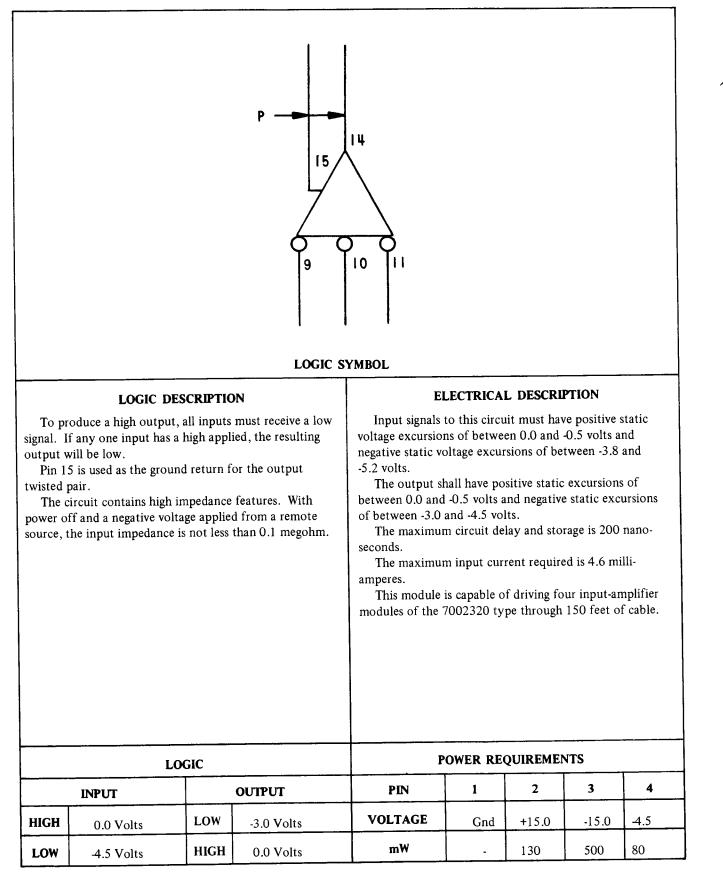
Figure 7-33. Control Line Amplifier, Card Type 7002331
