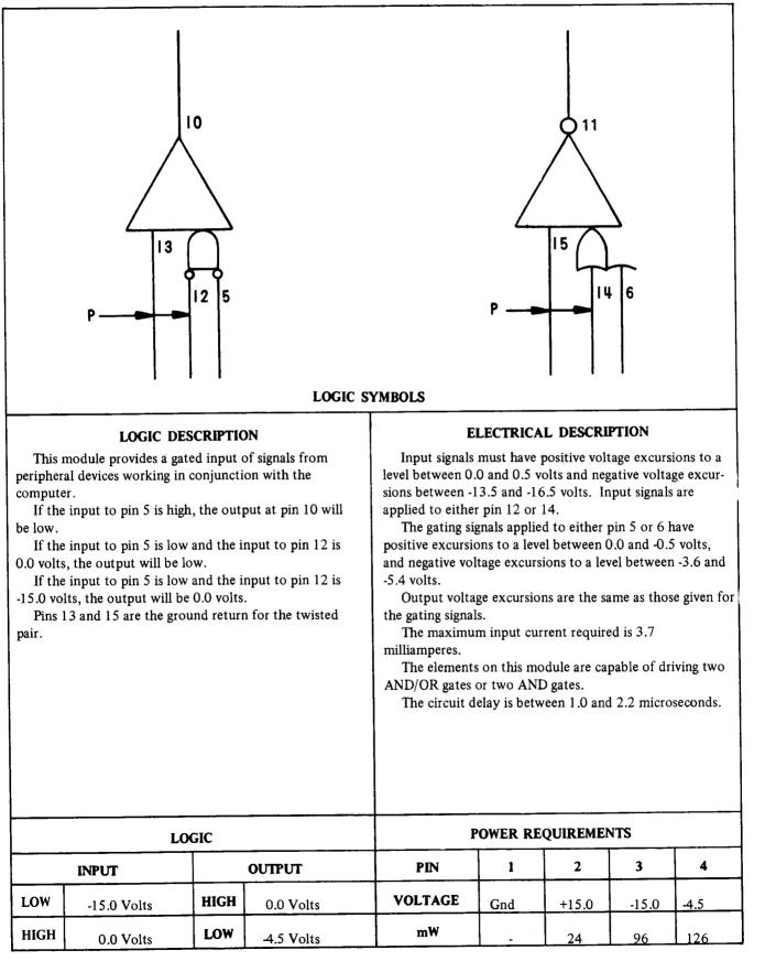
Figure 7-25. Input Amplifier-Inverter, Card Type 7002090
