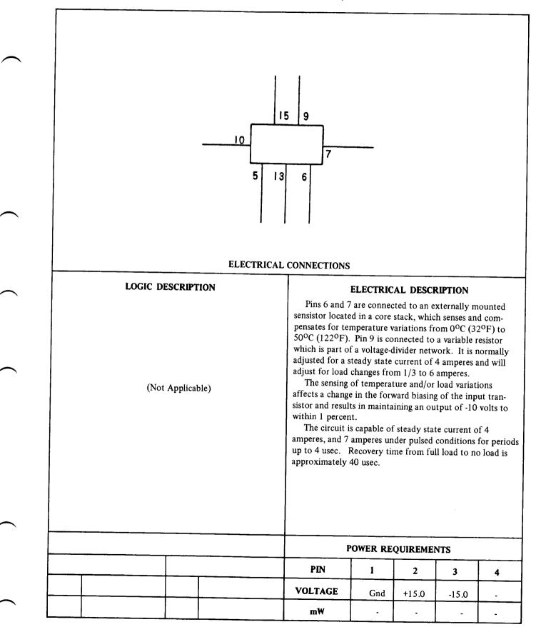
Figure 7-44. Regulator Amplifier (-10 volt), Card Type 7003600
