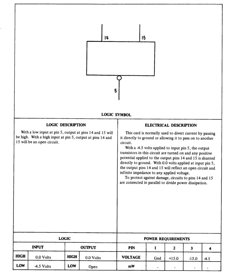
Figure 7-54. Current-Control Diverter, Card Type 7003760
