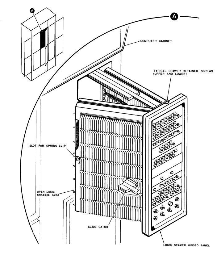
Figure 7-10. Extended Logic Drawer A2
