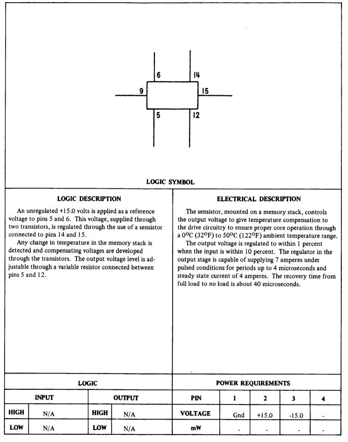
Figure 7-52. Regulator Amplifier (+10 volt), Card Type 7003730
