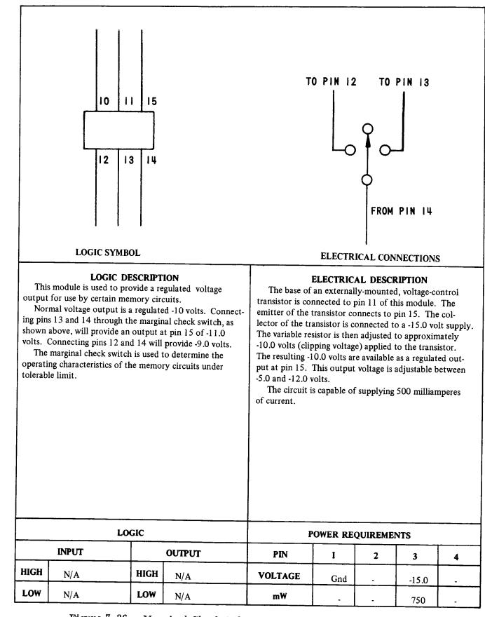
Figure 7-36. Marginal Check Voltage Regulator, Card Type 7002861
