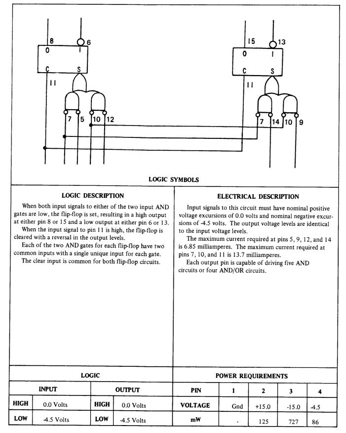
Figure 7-38. Flip-Flop, Card Type 7002900
