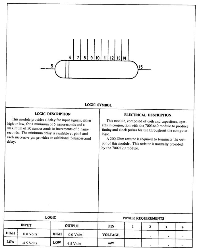
Figure 7-46. Pulse-Delay Network, Card Type 7003630
