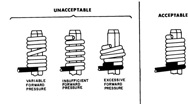
Figure 7-7. Wire-Wrap Connections
