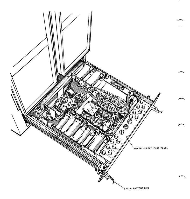
Figure 7-11. Extended Power Supply PS 1
