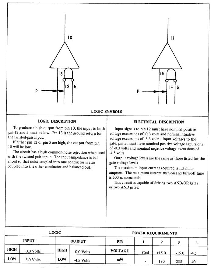
Figure 7-32. Differential Amplifier, Card Type 7002321
