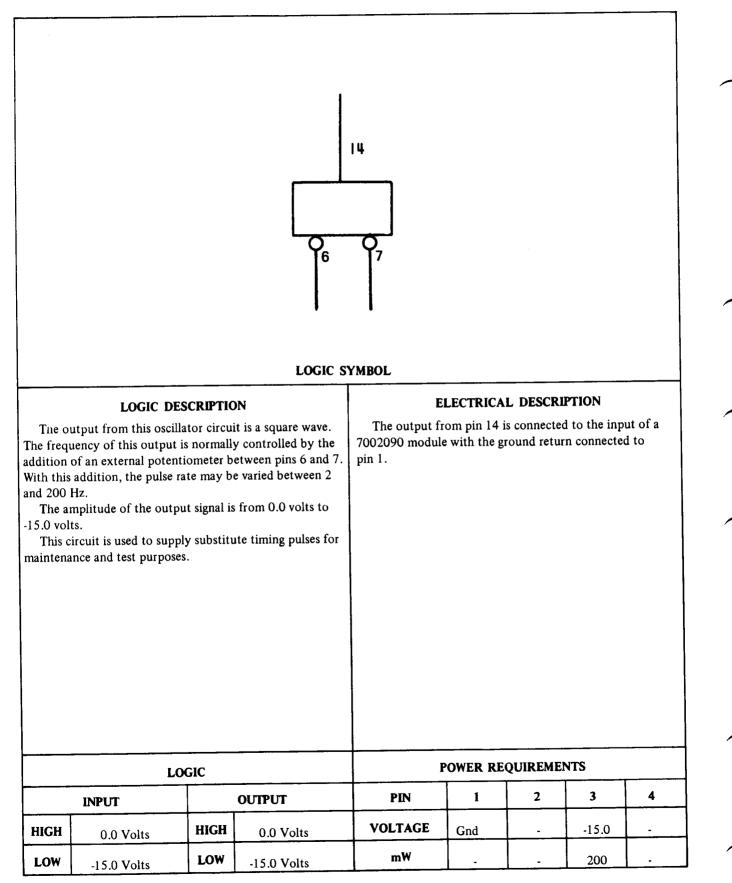
Figure 7-15. Pulse-Delay Oscillator, Card Type 7000210
