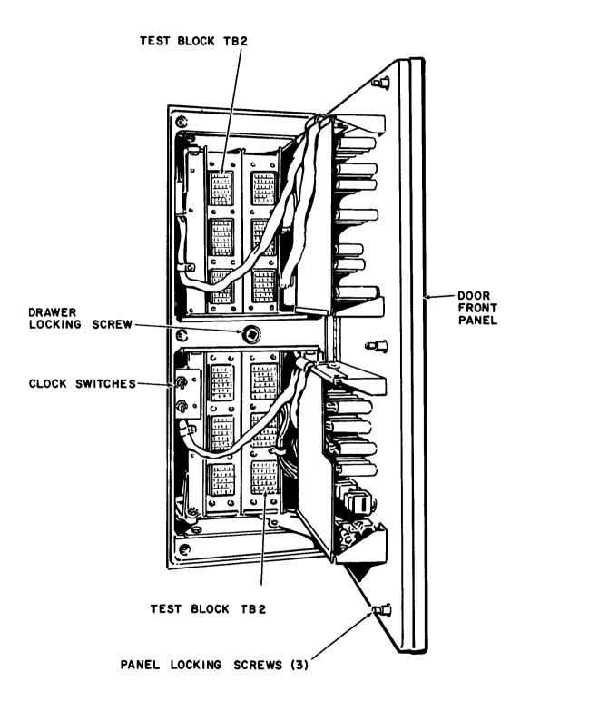
Figure 7-9. Location of Parts in Logic Drawer-Panel Opened
