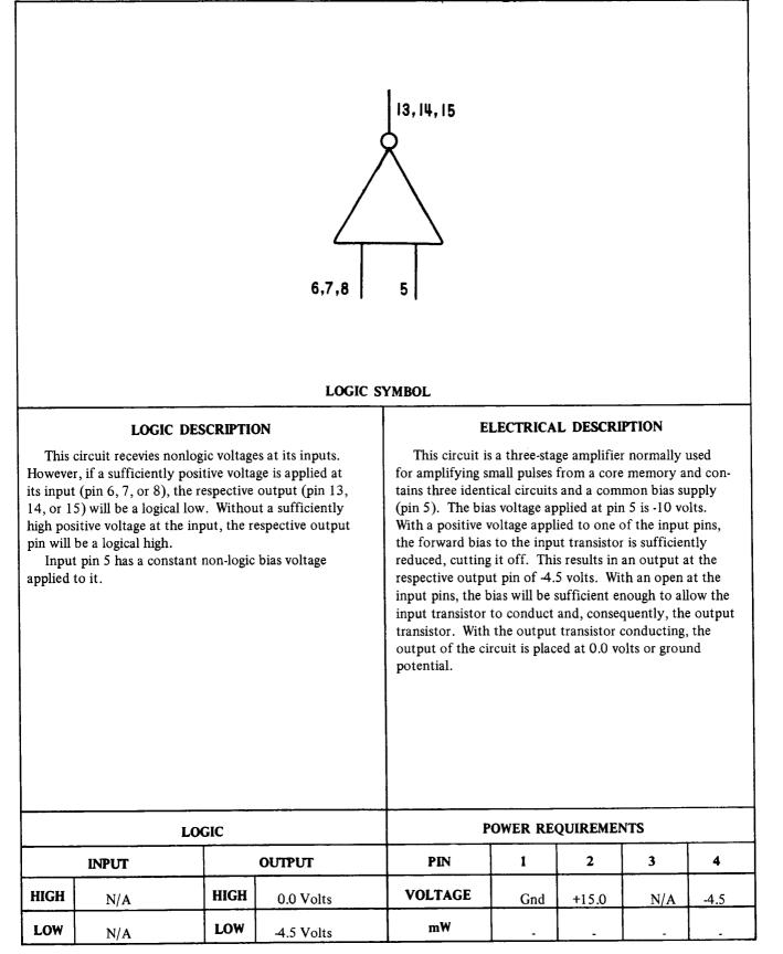
Figure 7-57. Output-Sense Amplifier, Card Type 7003850
