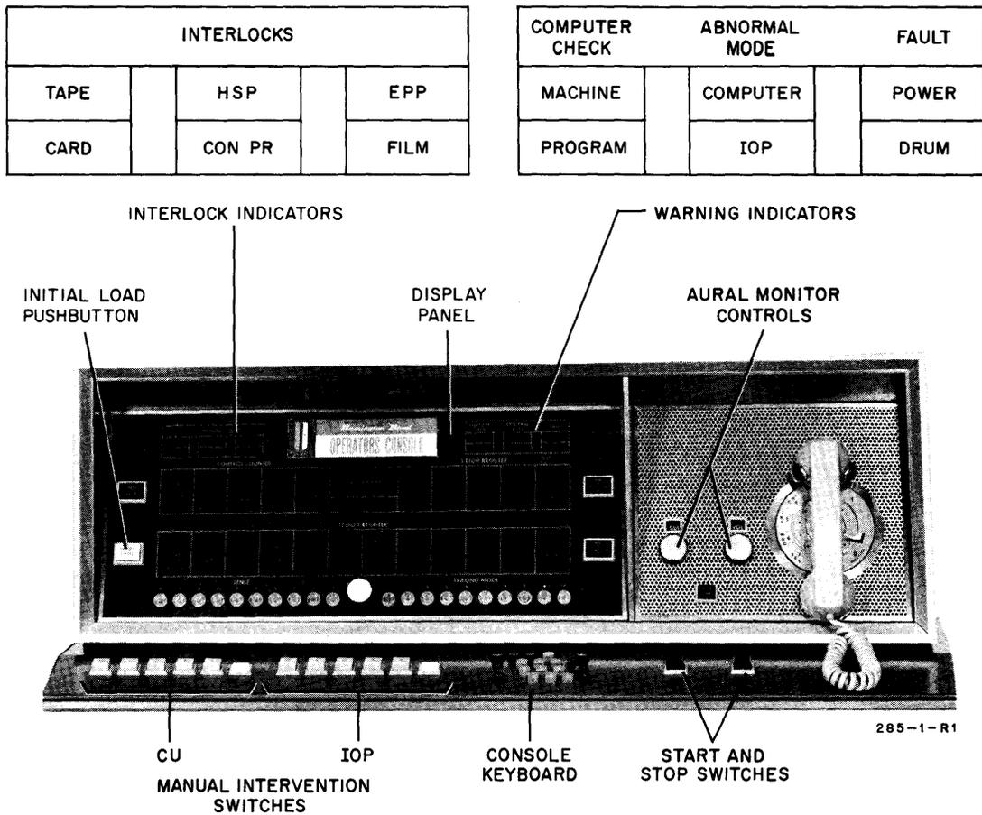
Figure 5-1. Operator's Console
