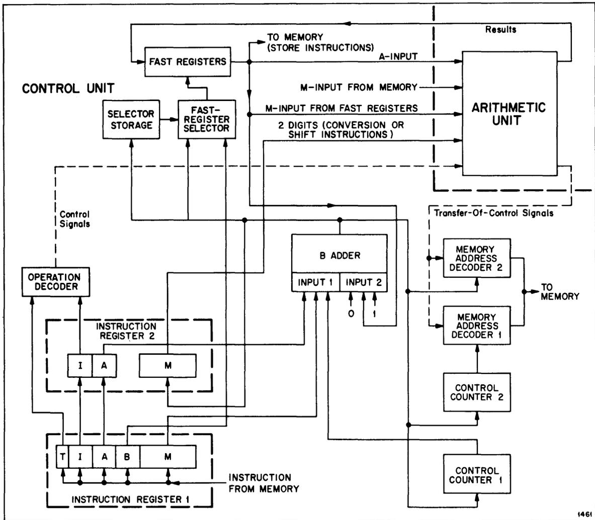
Figure 2-1. Computing Unit Block Diagram
