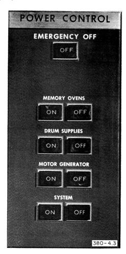
Figure 3-10. Power Control Panel
