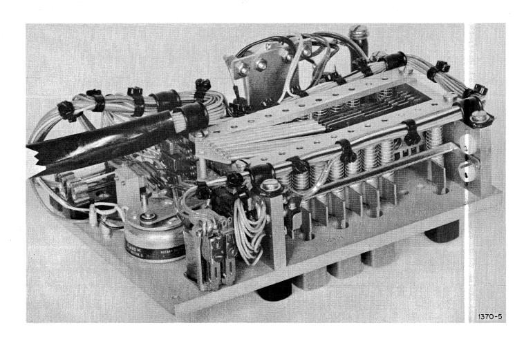
exercised in replacing the microswitch to avoid distortion of the microswitch bail. It should be noted that careful removal of the microswitch generally will not affect adjustment of the bail.
