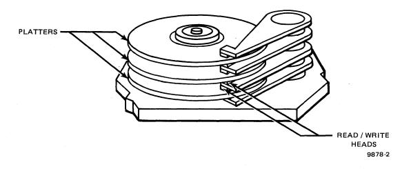
Figure 1–2. Disk Drive Assembly
