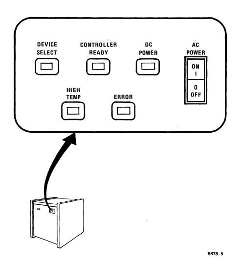
Figure 2–1. 8409 Disk Subsystem Front Panel Controls and Indicators
