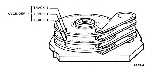
Figure 1-4. Disk Track and Cylinder Location
