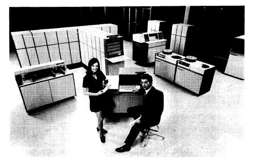
This view of a fairly small, disc-oriented UNIVAC 9700 configuration shows the CRT-equipped System Console in the foreground and the Central Processor at left rear.
