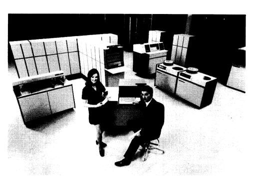
This view of a fairly small, disc-oriented UNIVAC 9700 configuration shows the CRT-equipped System Console in the foreground and the Central Processor at left rear.
