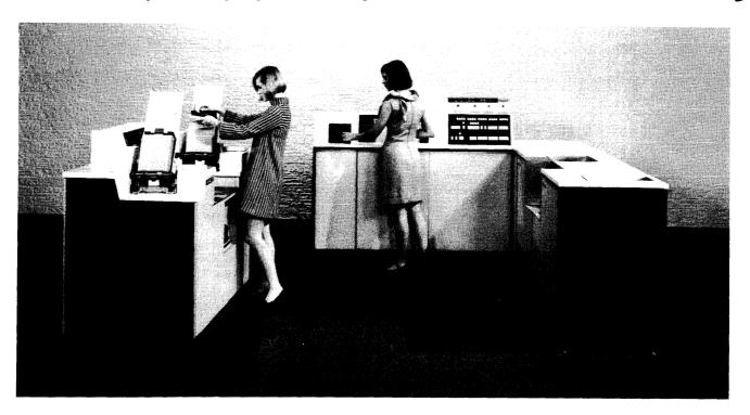
This card-oriented UNIVAC 9300 system includes the dual-feed 1001 Card Controller (left) as well as the basic card reader and
