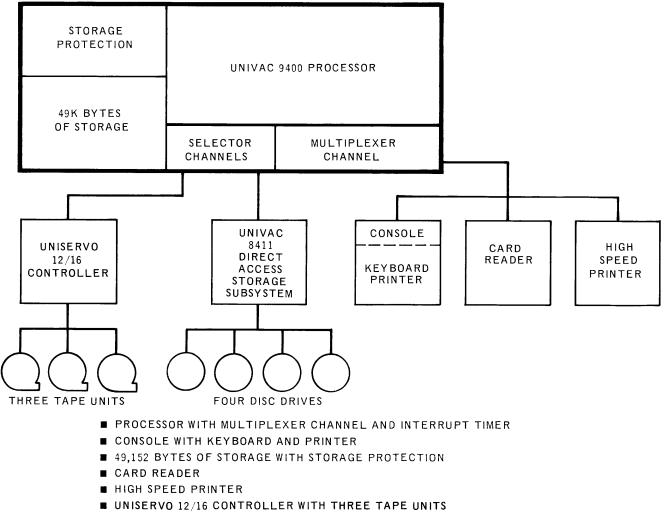
UNIVAC 8411 DIRECT ACCESS STORAGE SUBSYSTEM WITH FOUR DISC DRIVES
