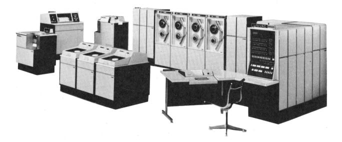
Figure 1-1. The UNIVAC 9400 System
