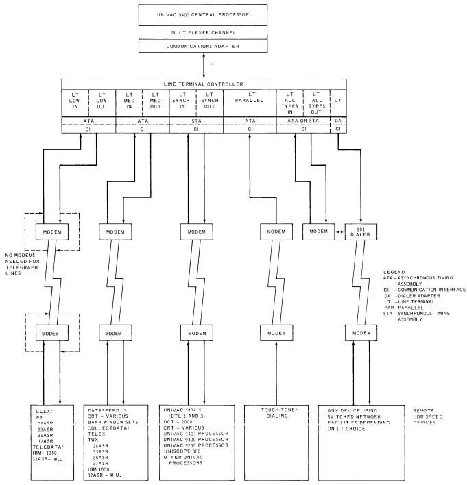
\* A SECOND UNIVAC 9400 CENTRAL PROCESSOR CAN BE CONNECTED TO THE DATA COMMUNICATION SUBSYSTEM (DCS-16) THROUGH THE USE OF THE DUAL CHANNEL ADAPTER. THIS CONNECTION IS MANUALLY SWITCHED AND ALLOWS ONLY ONE PROCESSOR AT A TIME TO INTERFACE WITH THE DATA COMMUNICATION SUBSYSTEM.
