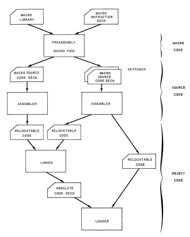
Figure 1-2. 9200/9300 Assembly System
