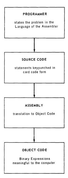
Figure 1-1. Source-to-Object Code Translation with Assembler
