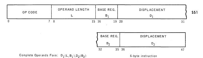
The instructions with this format are used to process data in storage where the operands are of equal length, and include such functions as comparing, transferring, translating, and logical operations. The mnemonic codes for instructions using this type of format are:
