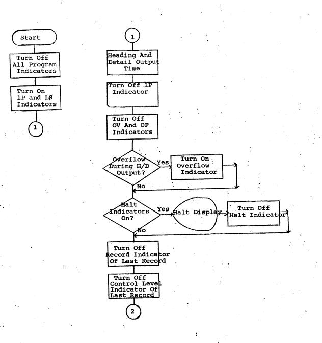
Figure 2-8. Operating Cycle Flowchart (Part 1 of 3)
