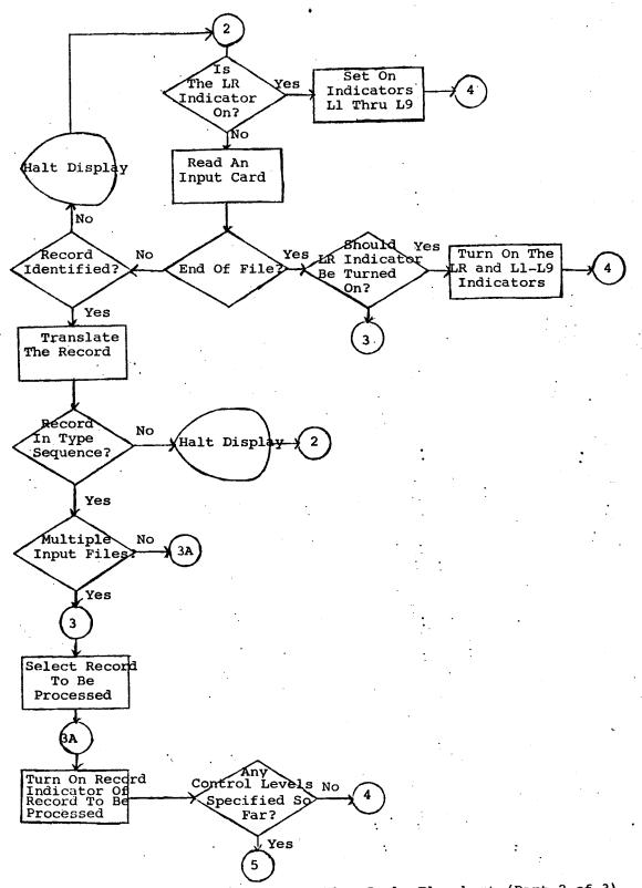
Figure 2-8. Operating Cycle Flowchart (Part 2 of 3)
