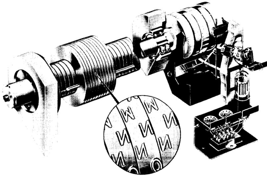
Figure 2-2. Printer Typewheels
