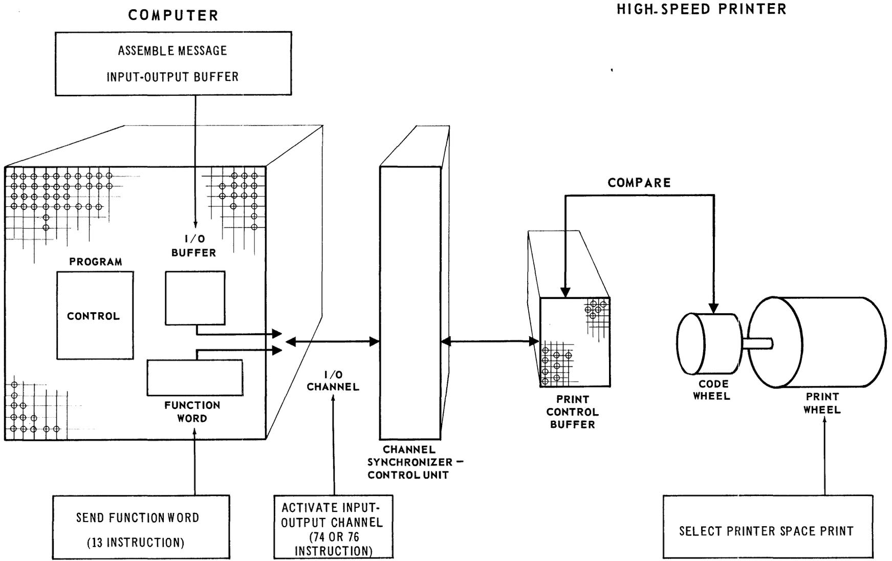
Figure 4-2. UNIVAC 490 Computer and the High-Speed Printer
