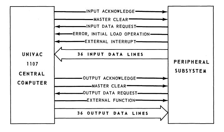
Figure 2-1. UNIVAC 1107 Input-Output Channel
