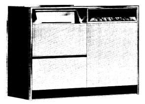
Figure 4-3. High-Speed Printer
