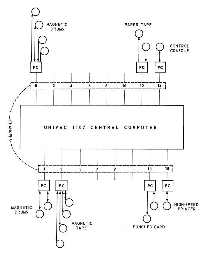
Figure 5-1. Typical UNIVAC 1107 Thin-Film Memory Computer System
