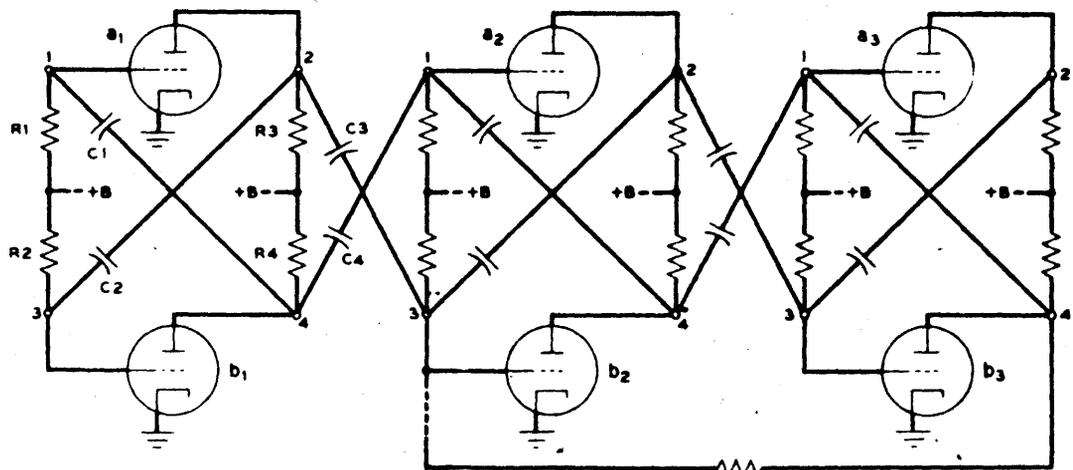
Fig. 3—Schematic of a three-stage multivibrator step-down
