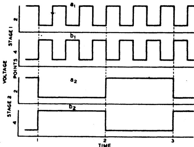
Fig. 4—Voltages across points 2 and 4 for the first few cycles of a multi-stage multivibrator step-down
