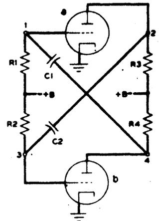
Fig. 1—Schematic of a multivibrator circuit capable of acting as a step-down
