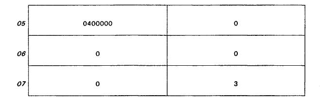
If H1 = 0400000 and H2 = 0, the location counter is nonexistent. Otherwise, a word of all zeros indicates a void location counter. The use of void location counters should be avoided since it makes the Collector less efficient. However, location counters 0 and 1 cannot be marked nonexistent.
