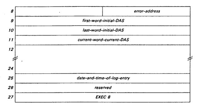
When a removable disk pack cannot be registered due to some unrecoverable error, the following log entry is created. The log format is shown in Table 9-31.
