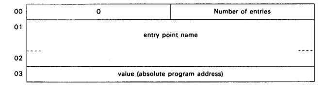
If the entry point is in a segment designated for indirect loading, H1 of word 3 contains the address of the entry for the entry point in the Indirect Load Table and H2 of word 3 contains the absolute program address of the entry point.
