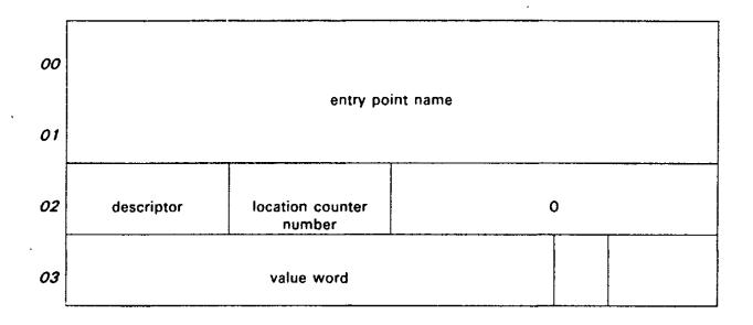
Each item is four words in length. The first two words contain the name of the entry point (LJSF Fieldata). The third word contains a descriptor, and the fourth word is a value word. Bit 27 of the third word is the type flag. If bit 27 is one, the entry point is absolute and has the value of the value word. If bit 27 is zero, the value word is relative to the location counter in bits 18 through 26. Entries in the entry point table need not be in any particular order.
