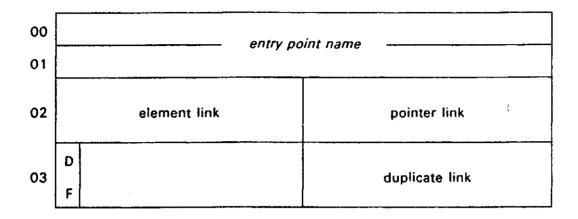
The element link is the sequence number of the element table item associated with the relocatable element containing the entry point.
