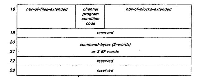
If the associated device type is mass storage, then the data in Words 18 through 23 have the following format:
