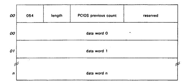
The end-of-reel (EOR) control record is inserted on an unlabeled tape after the end-of-tape (EOT) mark has been detected on a write.
