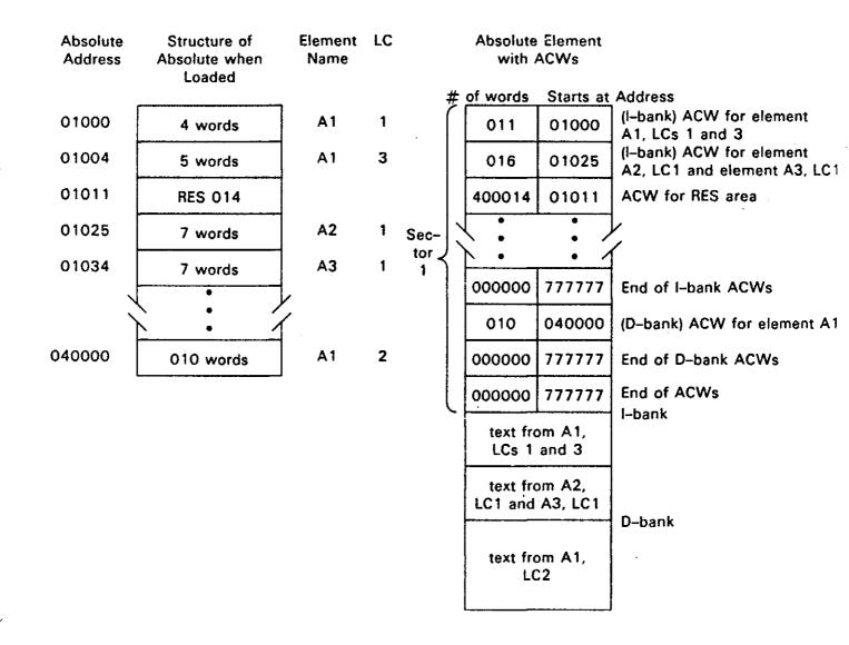
Bit 35 of the ACW, when set, tells the loader to zero fill the RES area.
