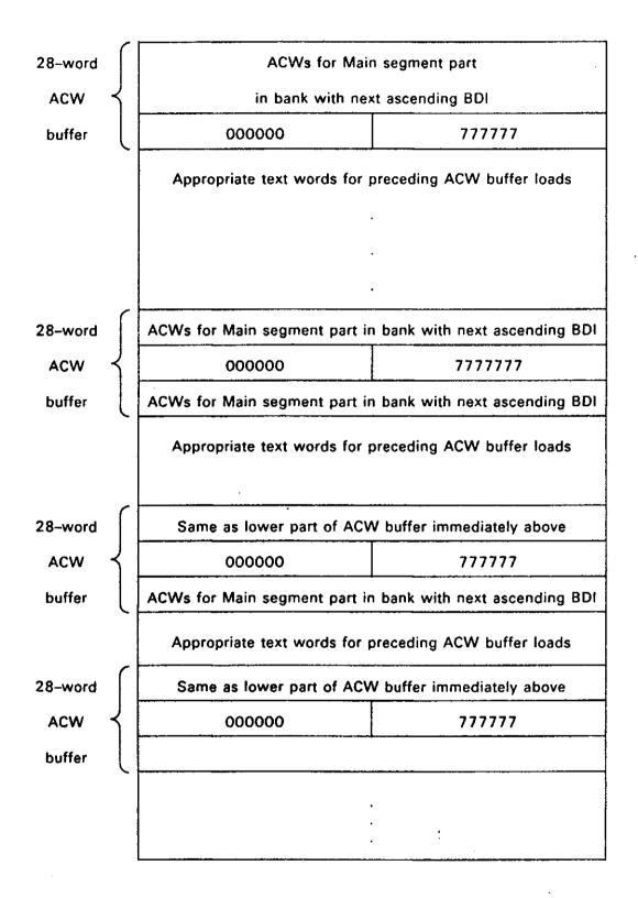
Figure 6-4. Main Segments in Initially Loaded Dynamic and Static Banks
