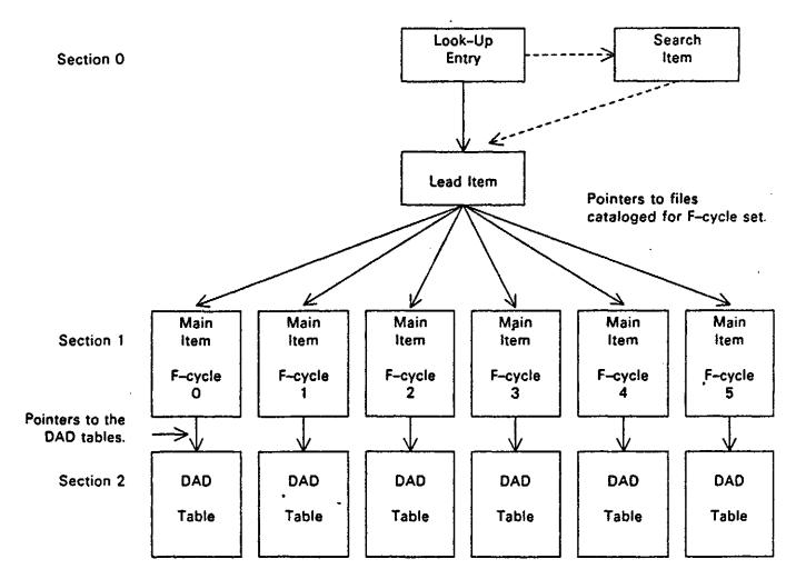
Figure 7-1. Example of an MFD Entry
