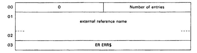
The external reference in the absolute text is assigned the address of the third word in XREF\$. Therefore, if a jump has been made to the external reference, an ER ERR\$ is done. This can be used for testing and debugging program modules.
