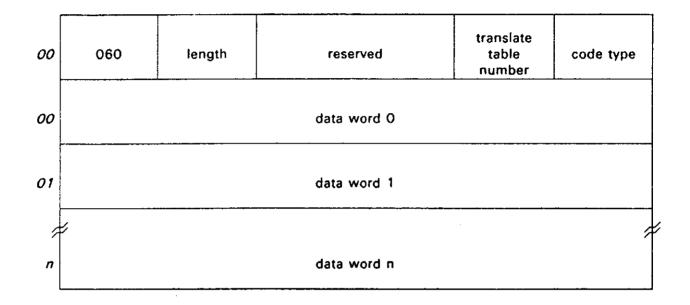
The ER PRTCN\$ control record consists of a control word with 060 in S1 and a special control record in the following several words. The special control word has the length of the special control record in S2 and the code type (1 for ASCII or 0 for Fieldata) in S6. The record consists of one or more print control functions to alter the printing of the file and has a maximum length of 63 words.
