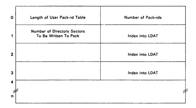
Thus, it can be seen that for removable disk, the device index points indirectly to the LDAT, via the user pack-id table. The user pack-id table resides in the Program Control Table (PCT) and contains one word for each pack assigned to the user.
