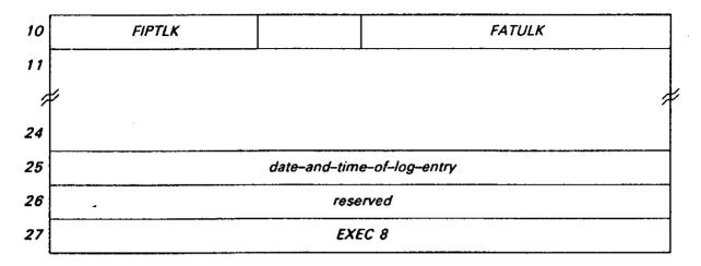
The log entry shown in Table 9–32 is created when a C/SP illegal function or communications error is encountered.
