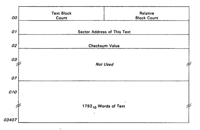
Text Block Count starts at zero and is incremented by one for every block copied on the tape for the file.
