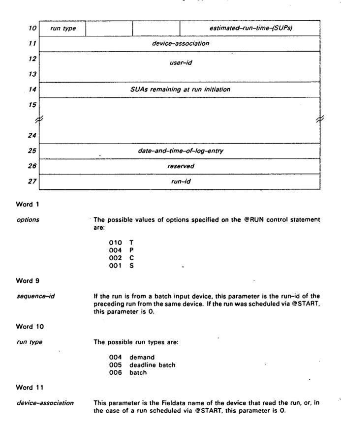
This entry is always the first one in the first block of a series of contiguous blocks in the master log file for a given run. The run-id field (new or generated) contains the same identity as Word 27 of each entry for the subject run.
