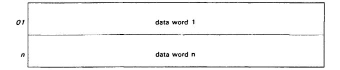
The end-of-file control record is used to indicate the end of actual file data. S1 of the control word contains 077. Any words in the file that follow this record are disregarded. Normal symbiont complex practice is to fill the last 224-word block to the end with end-of-file control records since the symbionts require the last block to be at least 224 words long. Tapes must have the last block equal to 224 or 1792 (0777 only) words in length.
