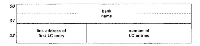
"Link address of first LC entry" is a word offset from the start of the LCT which describes the location counter.
