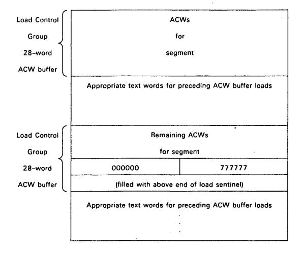
Figure 6-2. Example of Overlay Segments which Do Not Span Banks
