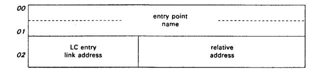
"LC entry link address" is the word offset from the start of the LCT which describes the location counter. Relative address is the address of the entry point relative to the start of the location counter. The Entry Point Name Table is created in alphabetical order.
