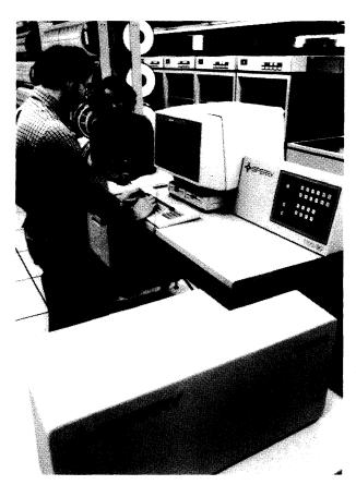
Unisys' 1100/90 SV models offer 1100/60 and 1100/70 users a lower entry point into the 1100/90 Series. The uniprocessor 1100/91 SV is rated at 5.5 MIPS, while the dual-processor 1100/92 SV is rated at 10.2 MIPS.
