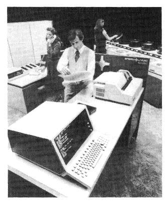
The 1100 60 system employs many peripherals announced for the original 1100 series. Included in this category are the Uniscope 200 and the terminal printer that are part of the systems console. The system support processor (SSP), a standard feature of the 1100 60 systems can support up to four consoles in a single processor configuration, or with the addition of a second SSP in a dual processor configuration, up to seven consoles.
