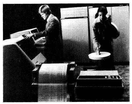
The DCP/40 is constructed with the same multi-microprocessor architecture as the 1100/60 processor. It can have over two million bytes of mainstorage and up to 16 I/O processors. Each I/O processor can control up to 16 communications lines. The DCP/40 is the hardware portion of the Teleon Intelligent Communications System.
