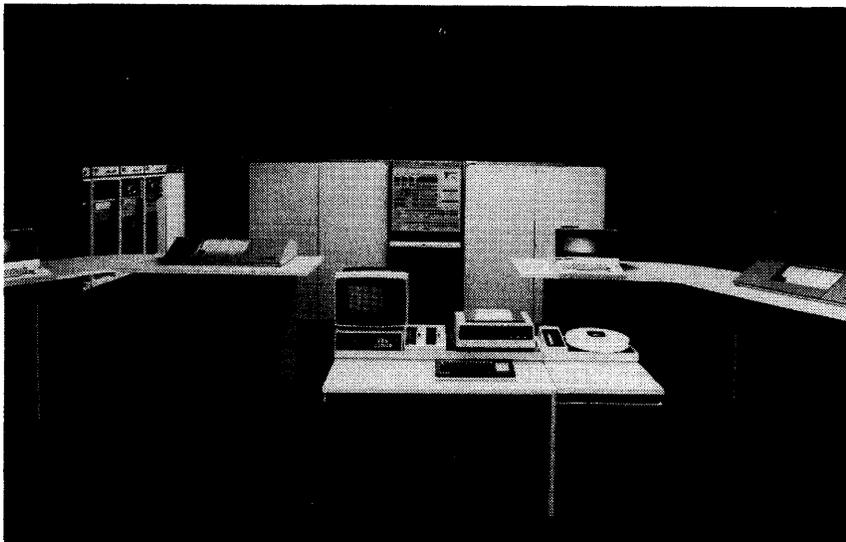
The Sperry Univac 1100/80 is the most powerful member of the 1100 Series family covered in this report. It is available in five distinct models: the low-end 1100/80, the single-processor 1100/81, the dual-processor 1100/82, the three-processor 1100/83, and the four-processor 1100/84.
