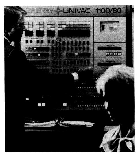
The Sperry 1100/80 System is available in a number of different configurations and offers a choice of system sizes ranging from one CPU to four CPUs. There are five 1100/80 models with multiprocessing capabilities an integral part of the systems. An array processor subsystem for processing large amounts of arithmetic data is also available.
