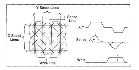
Coincident current core memory, four-wire arrangement and read/write current pulses.
