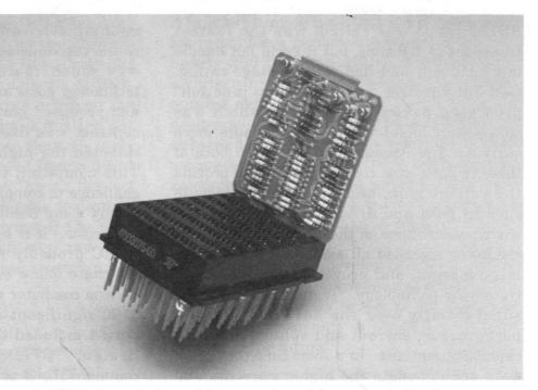
A 1107 logic card plugged into a section of the connector block.
