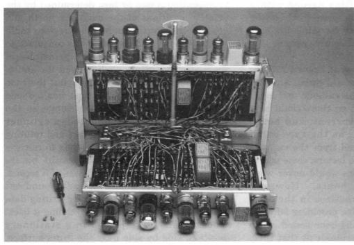
its output taken from the cathode rather than the usual plate). This isolated the output wiring load from the flip flop allowing it to change its state faster. The 1103 used about 12 types of tubes; the most common was the 5963 dual triode, an industrial version of the 12AU7, a common part in home television sets at the time.
