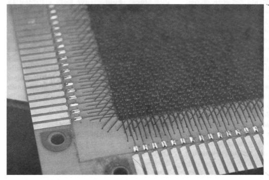
The 1107 was the first commercial computer to use a thin film memory. (MIT Lincoln Labs built a smaller one earlier). It represented payoff from about seven years of R and D when it was announced. Many companies other were also working on these types of memories. Film was a competitor to the core memory. It was made from a thin film of iron-nickel
