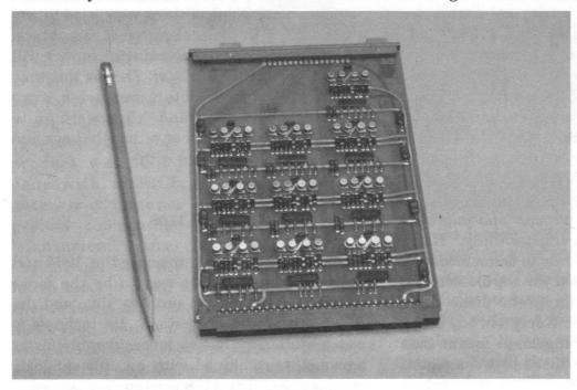
were needed, allowing a smaller, faster core. The cost of doing this was to require 36 sets of Y lines, one per bit, rather than only one set. The reduced cost of transistor drivers minimized the impact of this. Furthermore, each "plane" was made "non square" decreasing the number of Y lines per bit and increasing the X lines but minimizing the total number of drivers. This also reduced the back voltage on both X and
