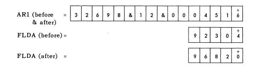
• Add the 5 least significant characters of arithmetic register 2 to the field labeled FLDA.
