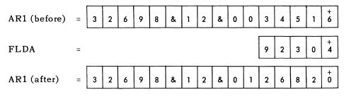
Add the five digit field labeled FLDA to arithmetic register 2.
