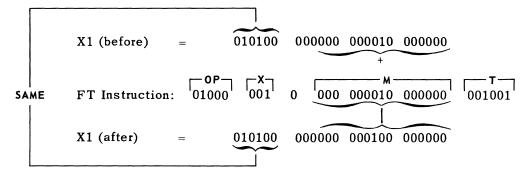
• Subtract the binary equivalent of a decimal 128 from the contents of index register 1.
