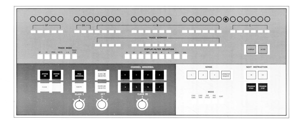
Figure 9-1. Central Processor Console
