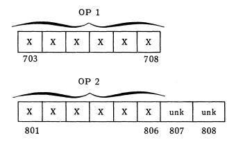
Instruction 2: Use the Transfer Constant (TK) Instruction to transfer space codes to the low-order positions of OP 2. (See Section 4.3.5 for a description of the TK instruction.) This will produce the desired result.
