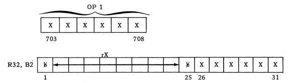
Instruction 2: Ascending Transfer specifying the LSL of rX (3231B2) as OP 1, LSL to the destination OP 2 (#801 - #808). The length of the OP 2 (8 locations) will cause the low-order 8 locations of rX to be transferred. This will produce the following results in OP 2.
