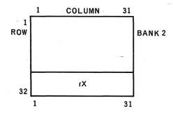
When the ICC is incremented for sequential access of instructions, it advances from R31/C31 of Bank 1, Bank 2, Bank 3, and Bank 4, to R1/C1 of Bank 2, Bank 3, Bank 4, and Bank 1 respectively, thus bypassing Row 32 and the special registers. The use of decimal addressing does not include the specification of the addresses of the Special Registers.
