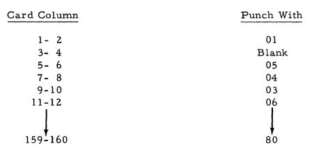
Will reproduce the card identically to the original except that Cols 3 and 5 will be punched into Cols. 5 and 3 and card column 2 will be blank.
