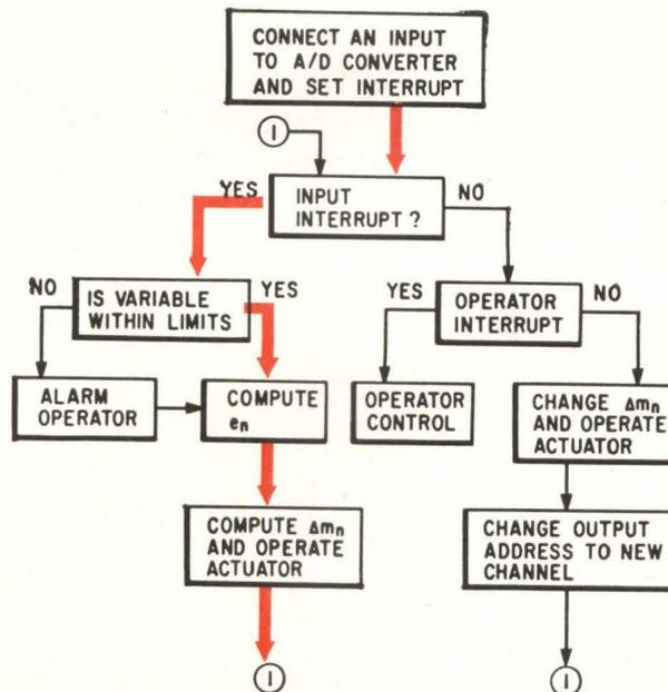
DDC computer operation is shown in this flow chart. Improved process control results from wider adjustment range and non-interacting parameters of signals
