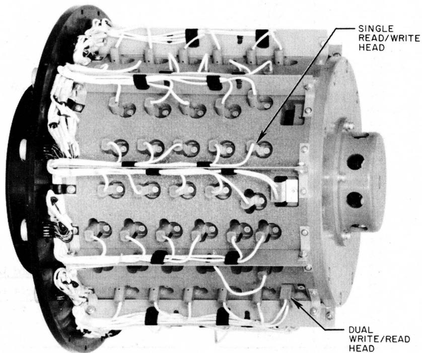
Figure 3-3. Drum Headmount Showing Location of Heads
