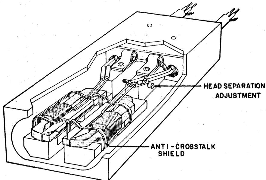
B. Dual Read and Write Head (One-word revolver)
