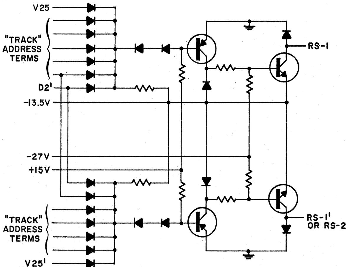
Figure 3-28. Relay Control Amplifier Pair, Schematic
