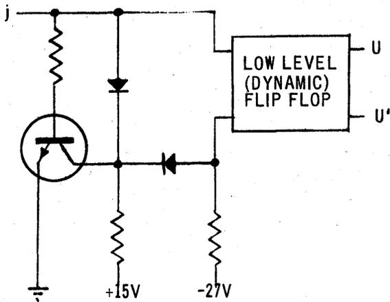
Figure 2-15. Delay Flip Flop, Simplified Diagram
