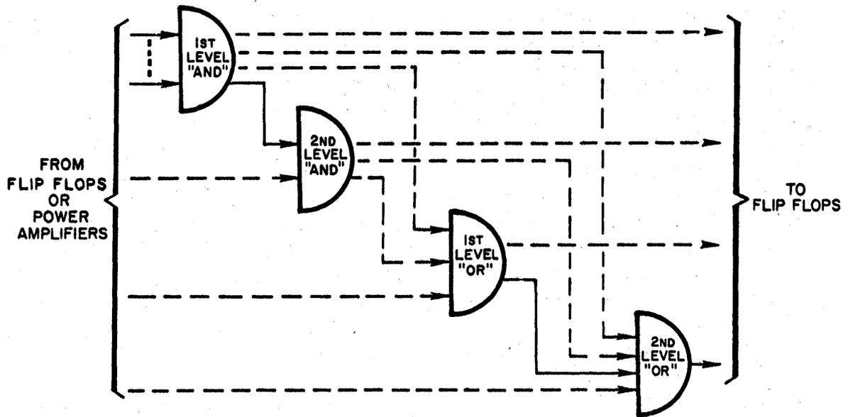
Figure 2-11. Two Level "And-Or" Gating (Required signal paths shown as solid lines; optional paths shown as dashed lines.)
