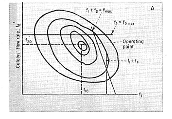
FIG. 6. Plots of constant profit in the  $f_1$   $f_2$  plane. A — Maximum operating profit realizable at  $(f_{10}, f_{20})$ ; B — Maximum operating profit not realizable at  $(f_{10}, f_{20})$ .
