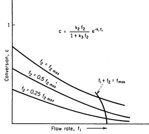
FIG. 4. Curves of conversion vs. flow rate  $f_1$  for three specific catalyst flow rates  $f_2$ .
