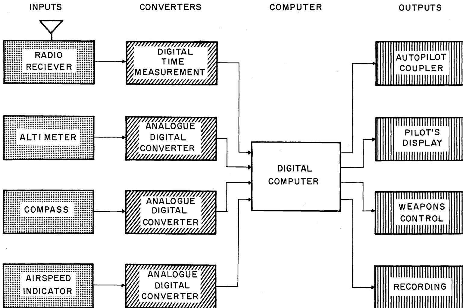
Fig. 3 Schematic Block Diagram of Digital Computer System for Performing Various Control Functions on Aircraft
