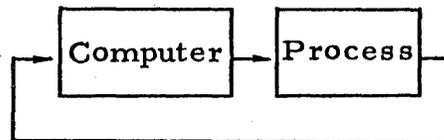
Fig. 2. Digital Control System - Feedback Type
