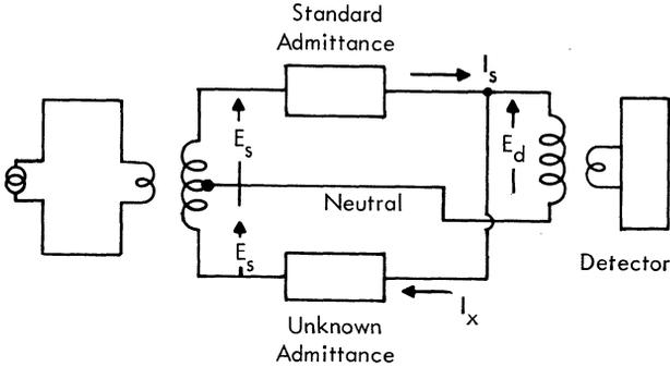
Fig. 7. Simplified diagram of Wayne Kerr bridge used for two-terminal measurements.
