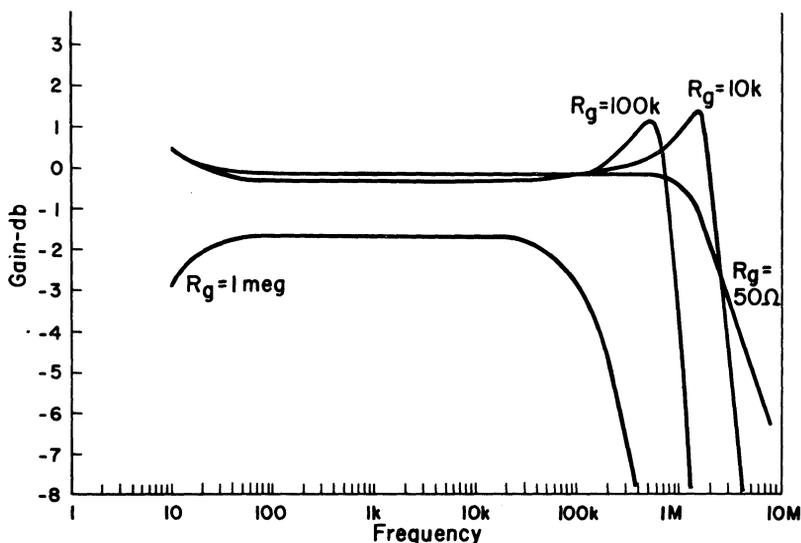
Fig. 15b. Frequency response curves of cascaded emitter follower.
