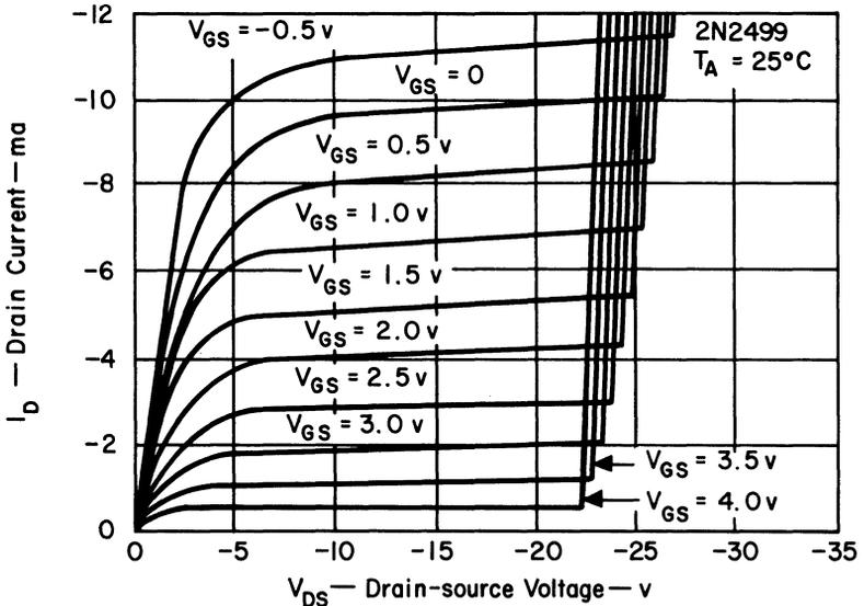
Fig. 13. Common-source drain characteristics.
