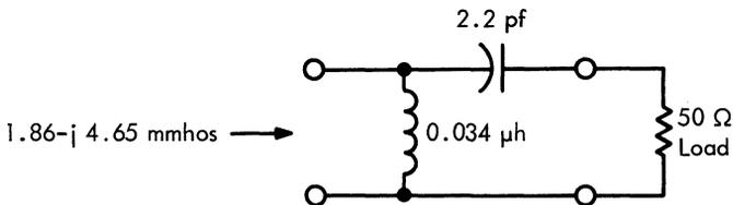
Fig. 3. Load resistance transforming network.
