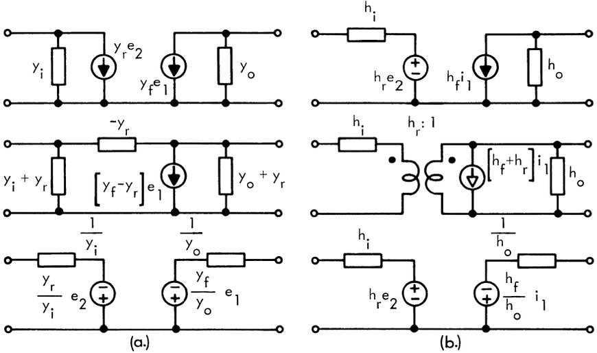
Fig. 2. One- and two-generator equivalent circuits in terms of: (a)  $y$  parameters; (b)  $h$  parameters.
