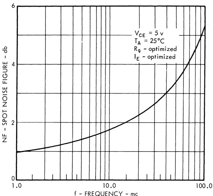
Fig. 3. Typical spot noise figure vs. frequency.
