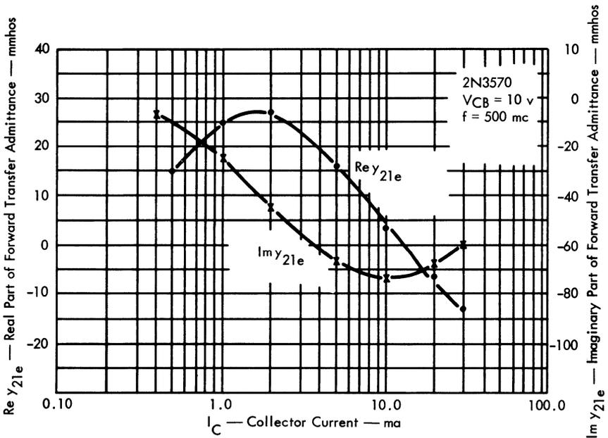
Fig. 1. 2N3570:  $\text{Re } y_{21e}$  and  $\text{Im } y_{21e}$  vs.  $I_C$ .
