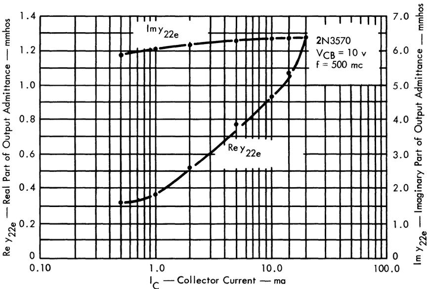
Fig. 4. 2N3570:  $\text{Re } y_{22e}$  and  $\text{Im } y_{22e}$  vs.  $I_C$ .
