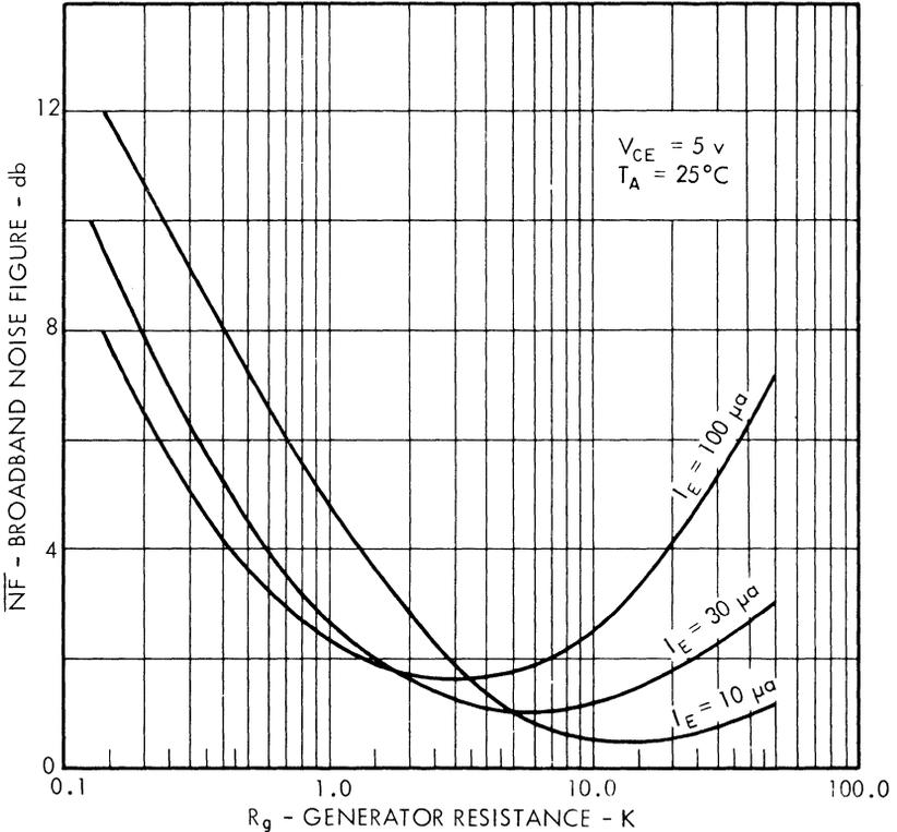
Fig. 1. Broadband noise figure vs. source impedance.
