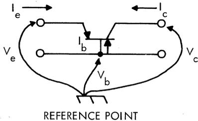
Fig. 3. A three-terminal network.
