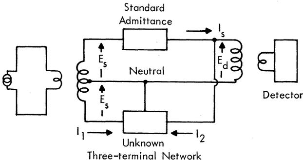
Fig. 8. Simplified diagram of Wayne Kerr bridge as used to measure the transfer admittance of a three-terminal network.
