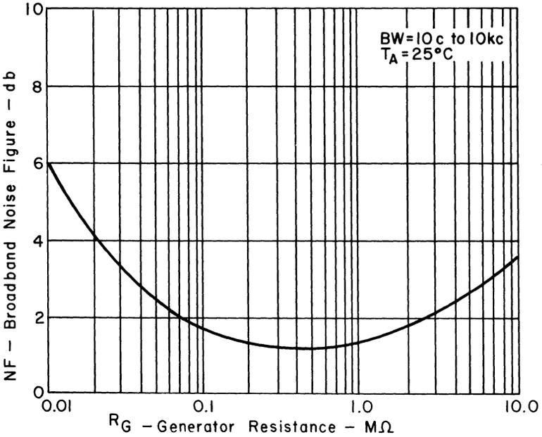
Fig. 47. Amplifier broadband noise figure vs. generator resistance.
