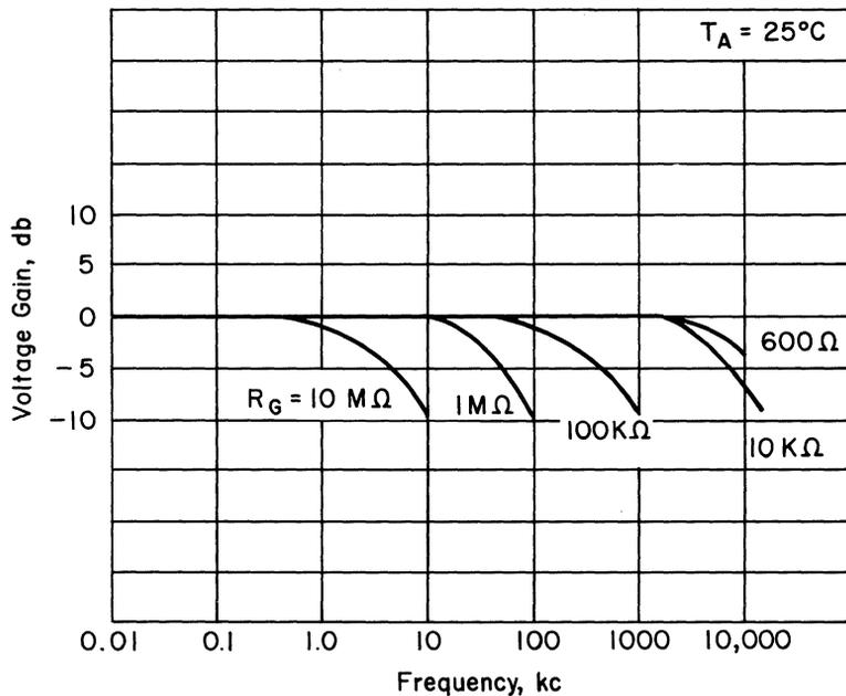
Fig. 42. Amplifier voltage gain vs. frequency.
