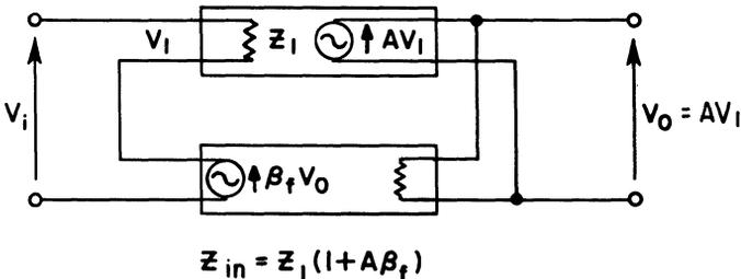
Fig. 2. Series-shunt connection.
