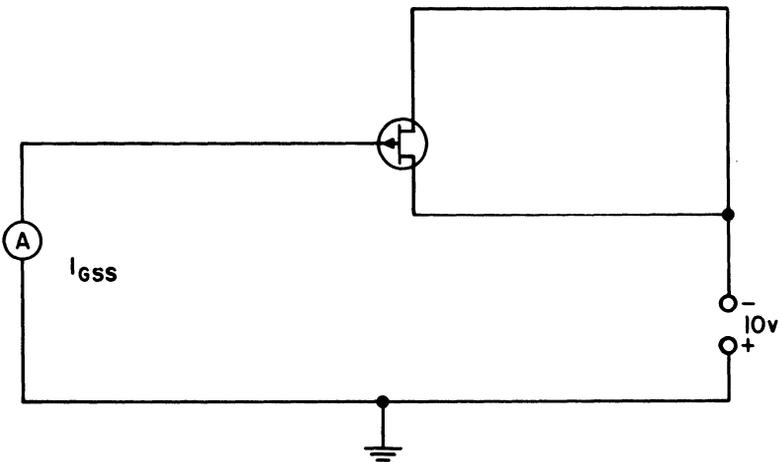
**Fig. 9. Gate cutoff current test circuit.**
