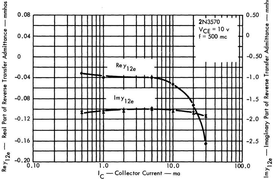
Fig. 5. 2N3570:  $\text{Re } y_{12e}$  and  $\text{Im } y_{12e}$  vs.  $I_C$ .
