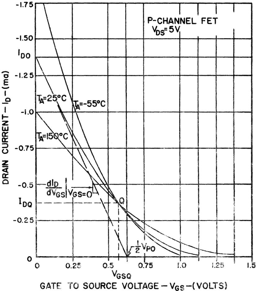
Fig. 2. Transfer characteristics with zero crossing.
