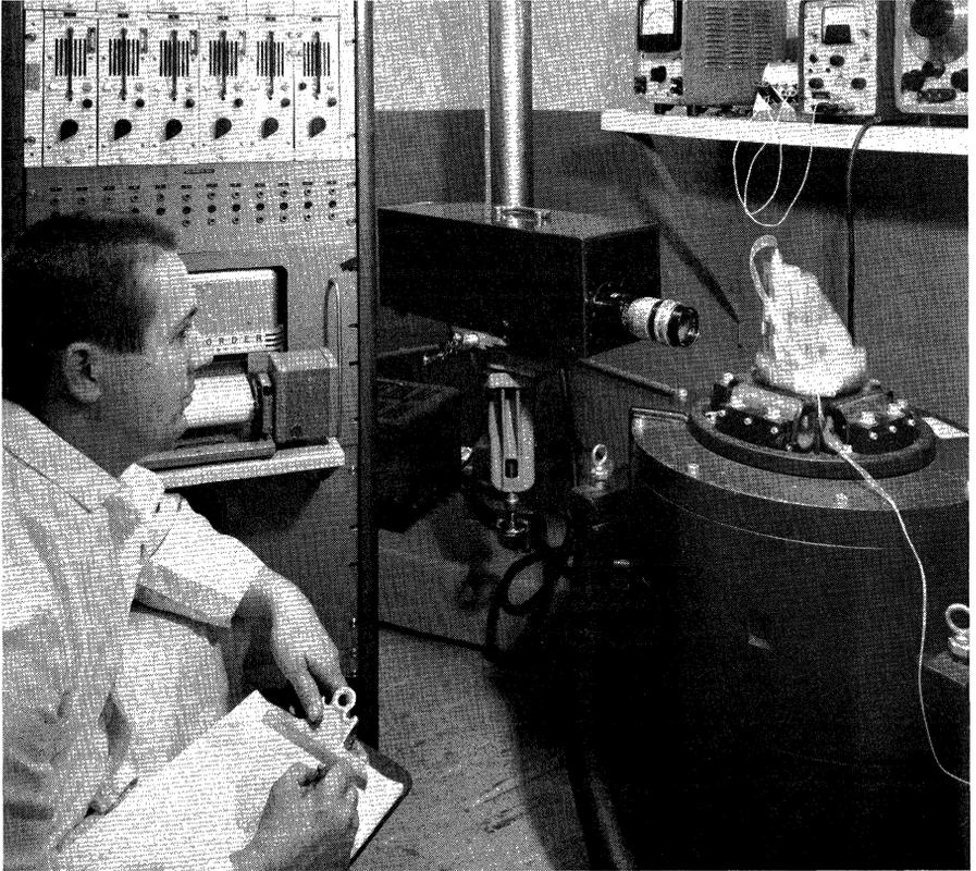
**Vibration table and displacement recorder in TI's Environmental Test Laboratory, one of the most extensive facilities of its kind in the world.**
