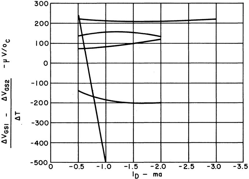
Fig. 27. Differential gate voltage tracking vs. drain current.
