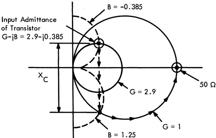
Figure 9. Input circuit design.
