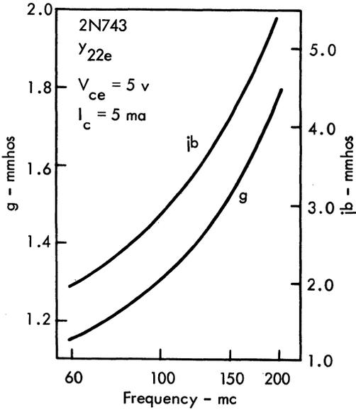
Fig. 6.  $y_{22e}$  vs. frequency (typical data).
