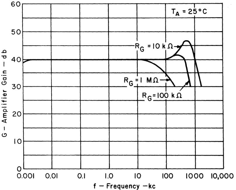
Fig. 48. Amplifier gain vs. frequency
