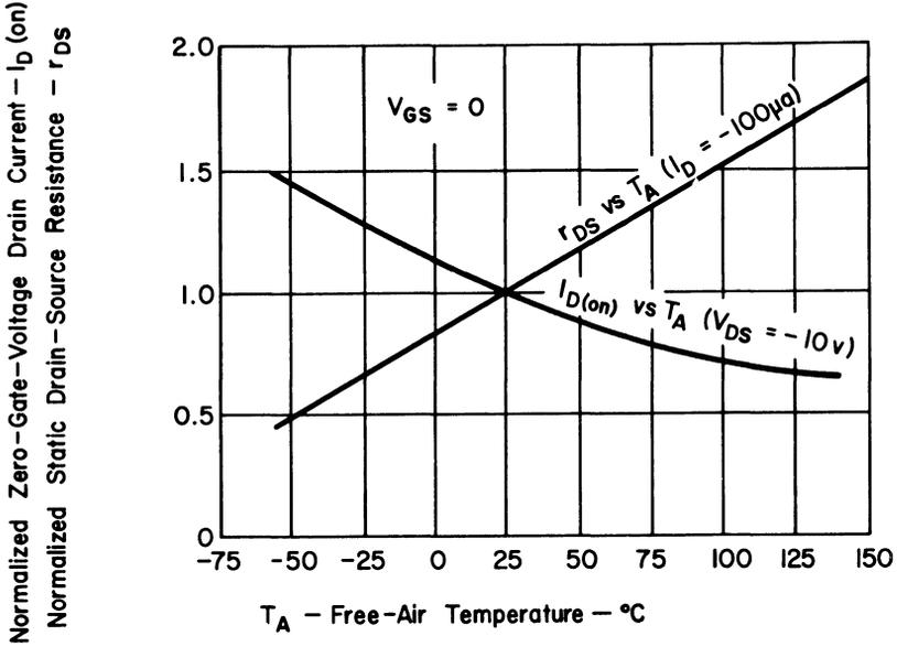
Fig. 16. Normalized zero-gain-voltage drain current and static drain-source resistance vs. free-air temperature.
