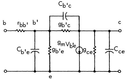
Fig. 1. Hybrid- $\pi$  equivalent circuit.
