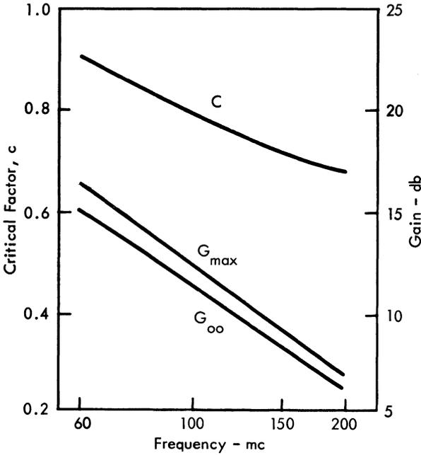
Fig. 7. 2N743 common-emitter, critical factor, and gain vs. frequency.
