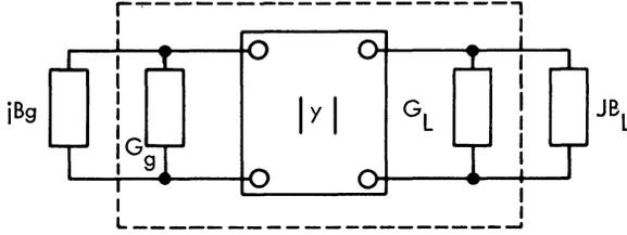
Fig. 13. Model used to demonstrate Stern's K factor.
