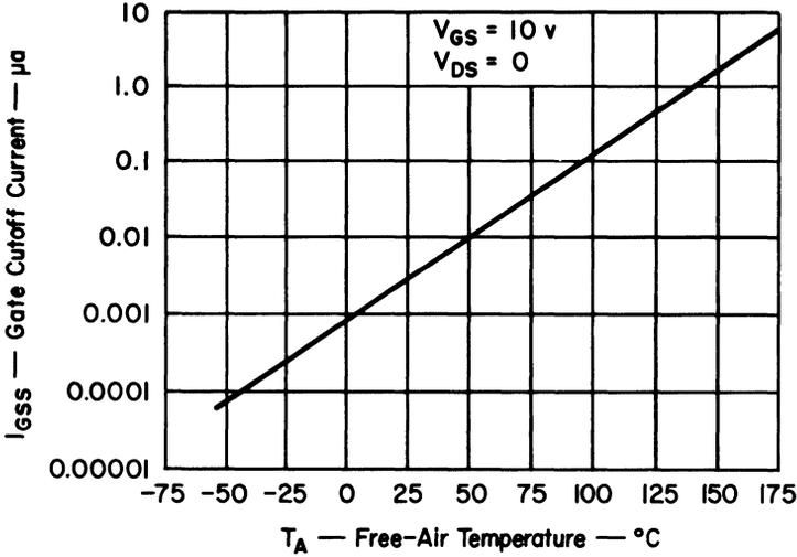
Fig. 10. Gate cutoff current vs. free-air temperature.
