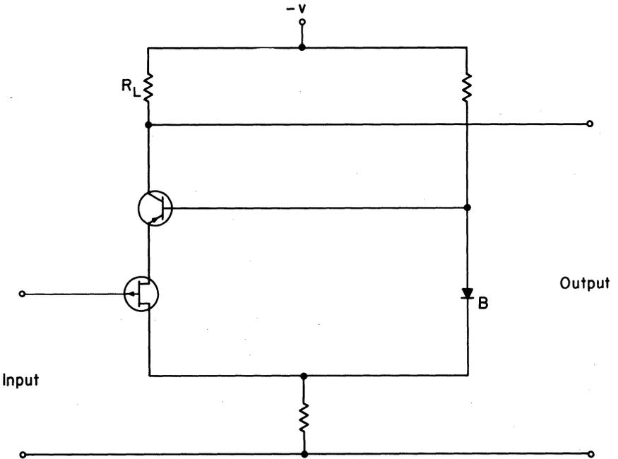
Fig. 40. Direct-coupled cascode circuit.
