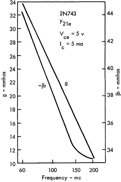
Fig. 5.  $y_{21e}$  vs. frequency (typical data).
