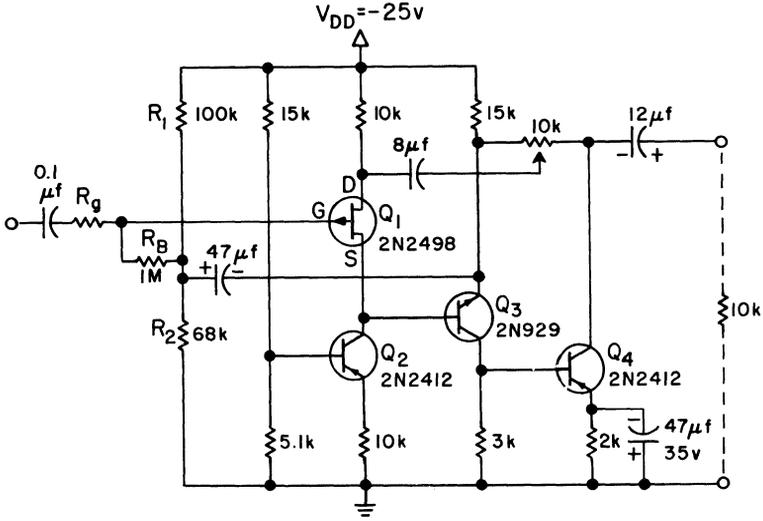
Fig. 21. 6-dB high input Z FET amplifier.
