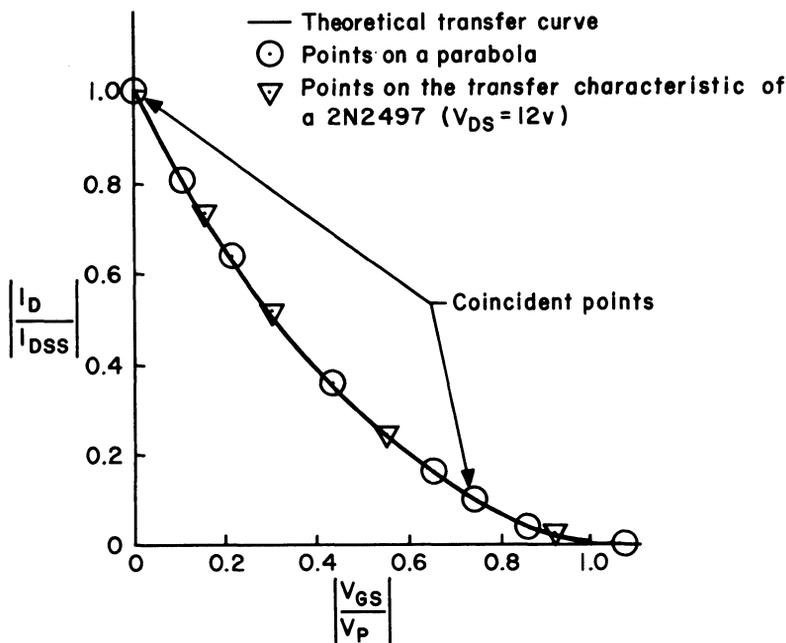
Fig. 8. Approximating the transfer curve with a parabola.
