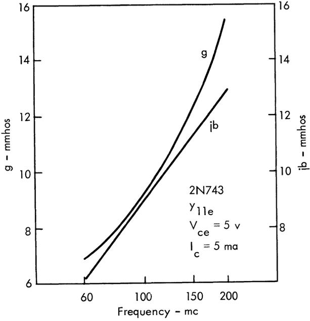
Fig. 3.  $y_{11e}$  vs. frequency (typical data).
