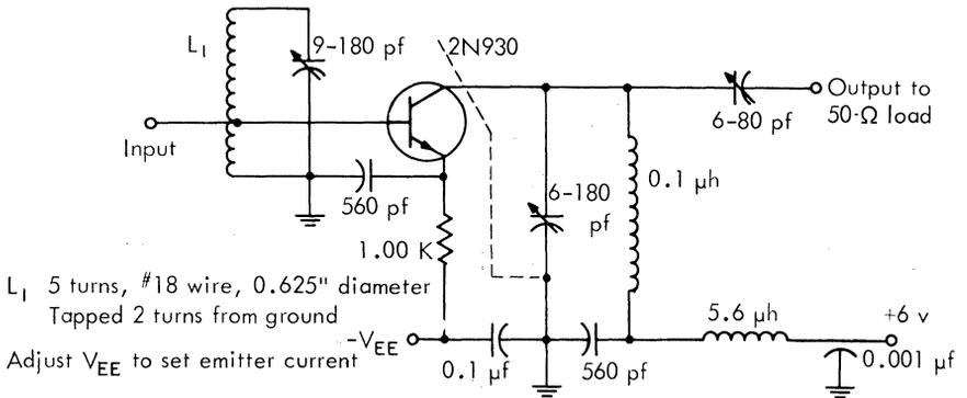
Fig. 5. 70-mc noise test amplifier.
