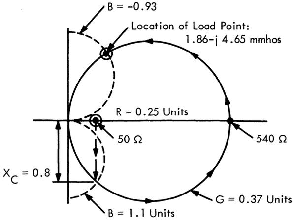
Fig. 2. Impedance-admittance chart for output network.
