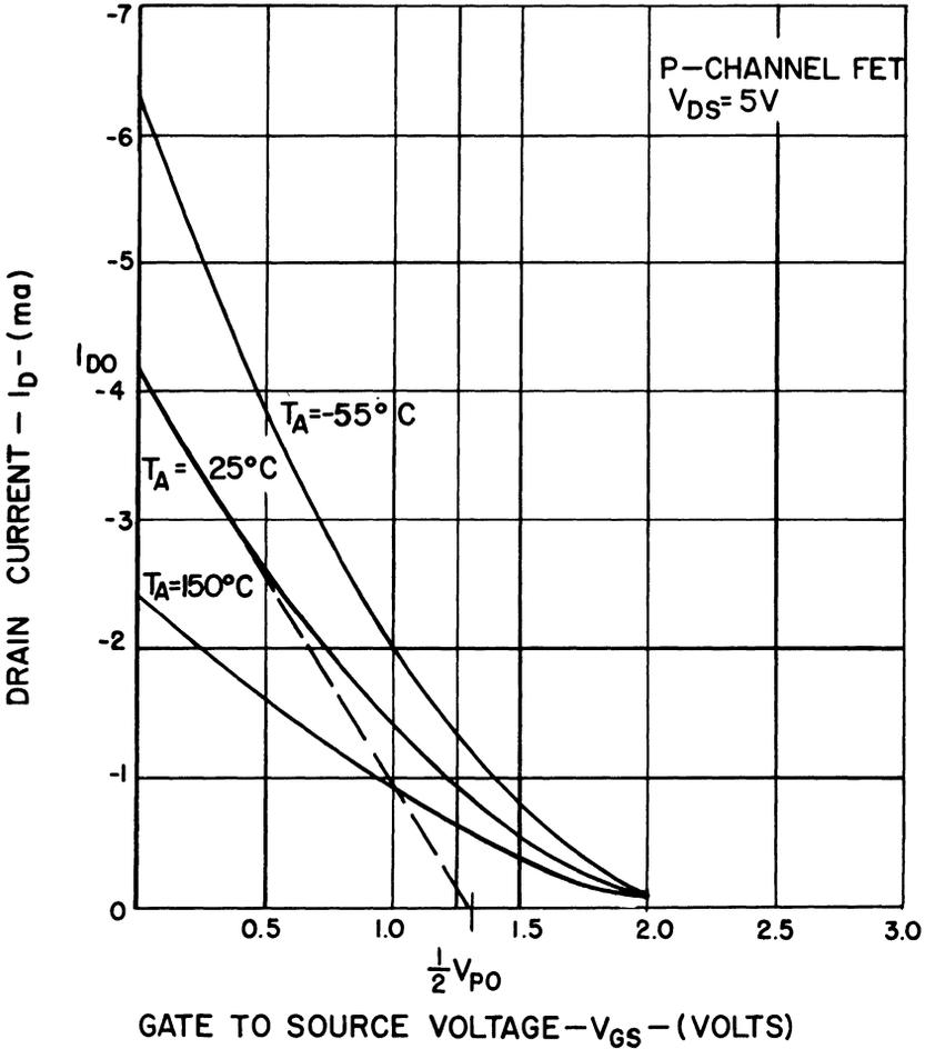
Fig. 3. Transfer characteristic with negative coefficient.
