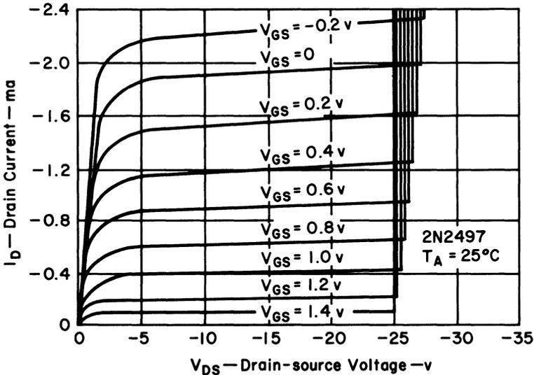
Fig. 11. Common-source drain characteristics.
