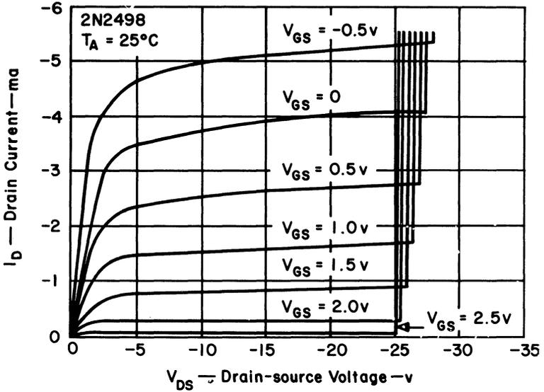
Fig. 12. Common-source drain characteristics.
