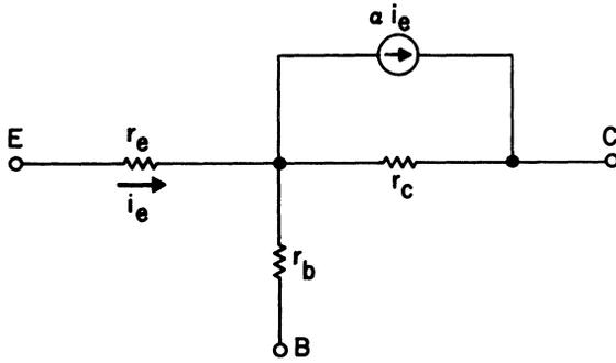
**Fig. 4. Common-base T-equivalent circuit.**
