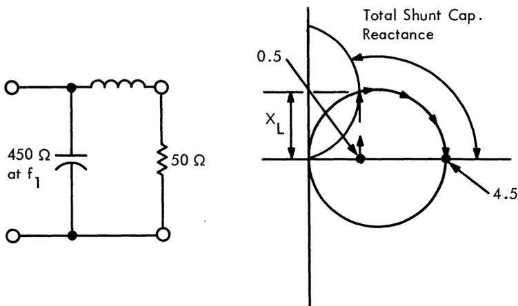
**Fig. 21. Series inductance L-section.**
