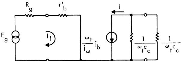
Fig. 5. High-frequency simplified equivalent circuit neglecting reverse internal feedback.
