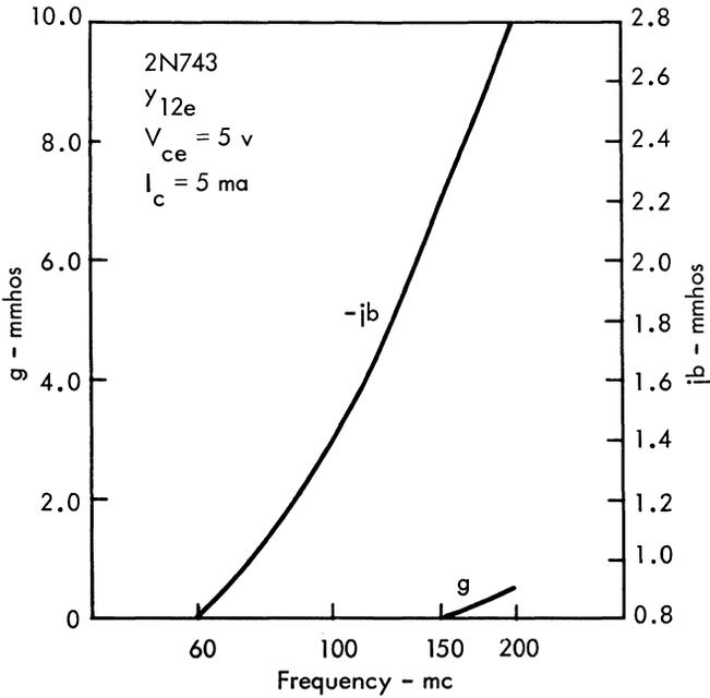
Fig. 4.  $y_{12e}$  vs. frequency (typical data).
