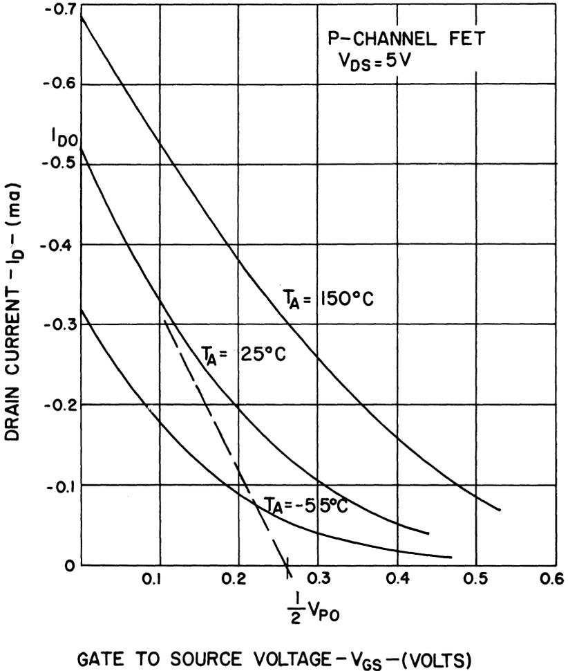
**Fig. 4. Transfer characteristic with positive coefficient.**
