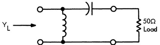
**Fig. 1. Load resistance transforming network.**
