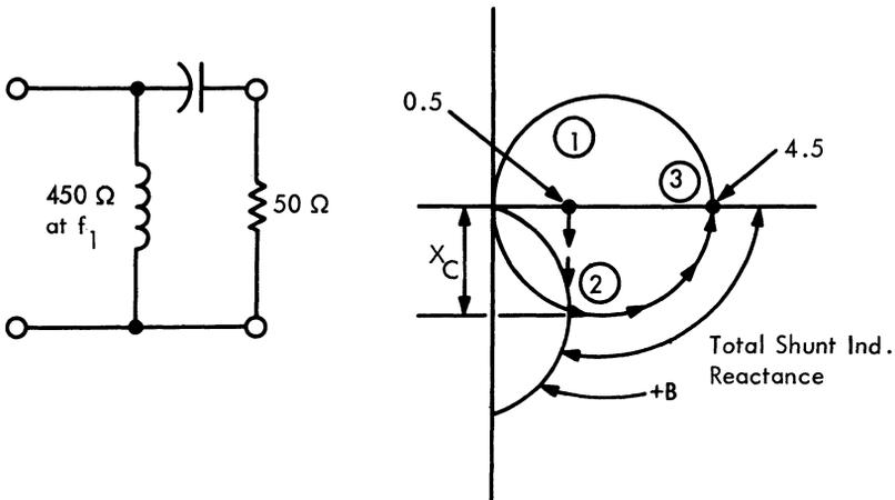
Fig. 20. Series capacitance L-section.
