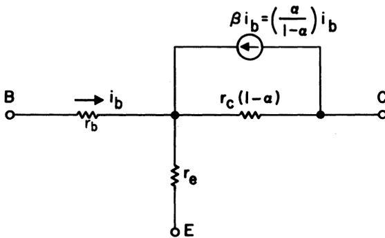
**Fig. 5. Common-emitter T-equivalent circuit.**
