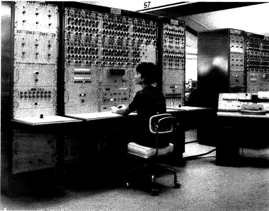
**"SMART,"** the TI-developed and TI-built Sequential Mechanism for Automatic Recording and Testing. Each SMART automatically measures 16 parameters in a few seconds, recording the data on punched cards.
