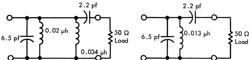
Fig. 4. Complete output network.
