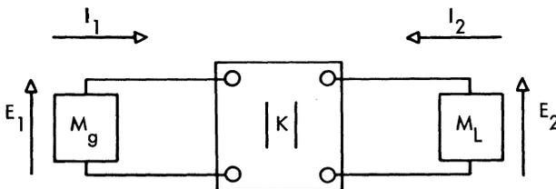
Fig. 9. A general active two-terminal pair with no external signal.
