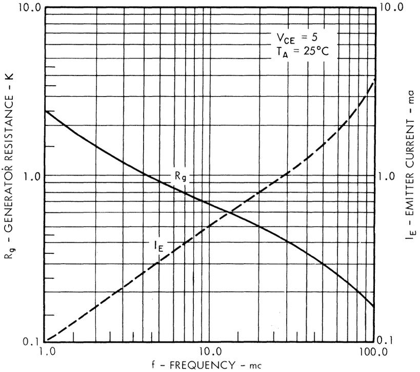
Fig. 4. Optimum source impedance and emitter current vs. frequency.
