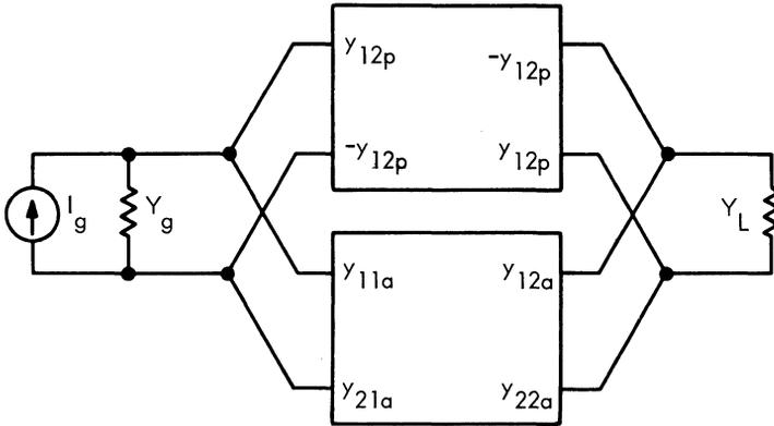
Fig. 2. A neutralized two-port.
