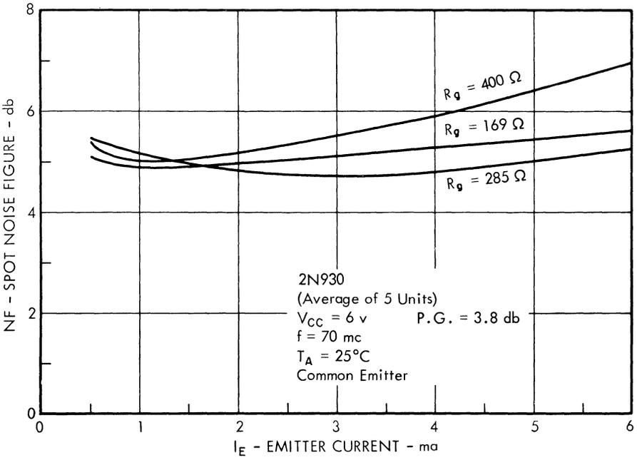
Fig. 6. Spot noise figure vs.  $I_E$  and  $R_g$ .
