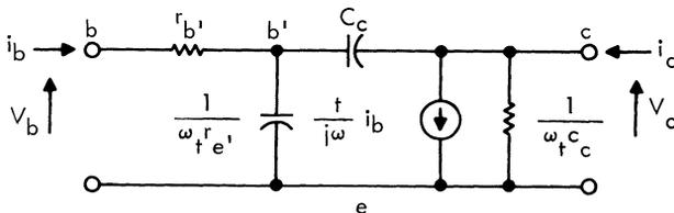
Fig. 2. Approximate high-frequency equivalent circuit of a junction transistor.
