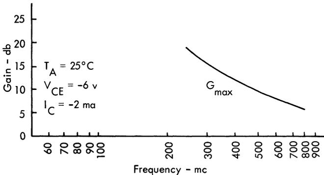
Fig. 4.  $G_{max}$  versus frequency.
