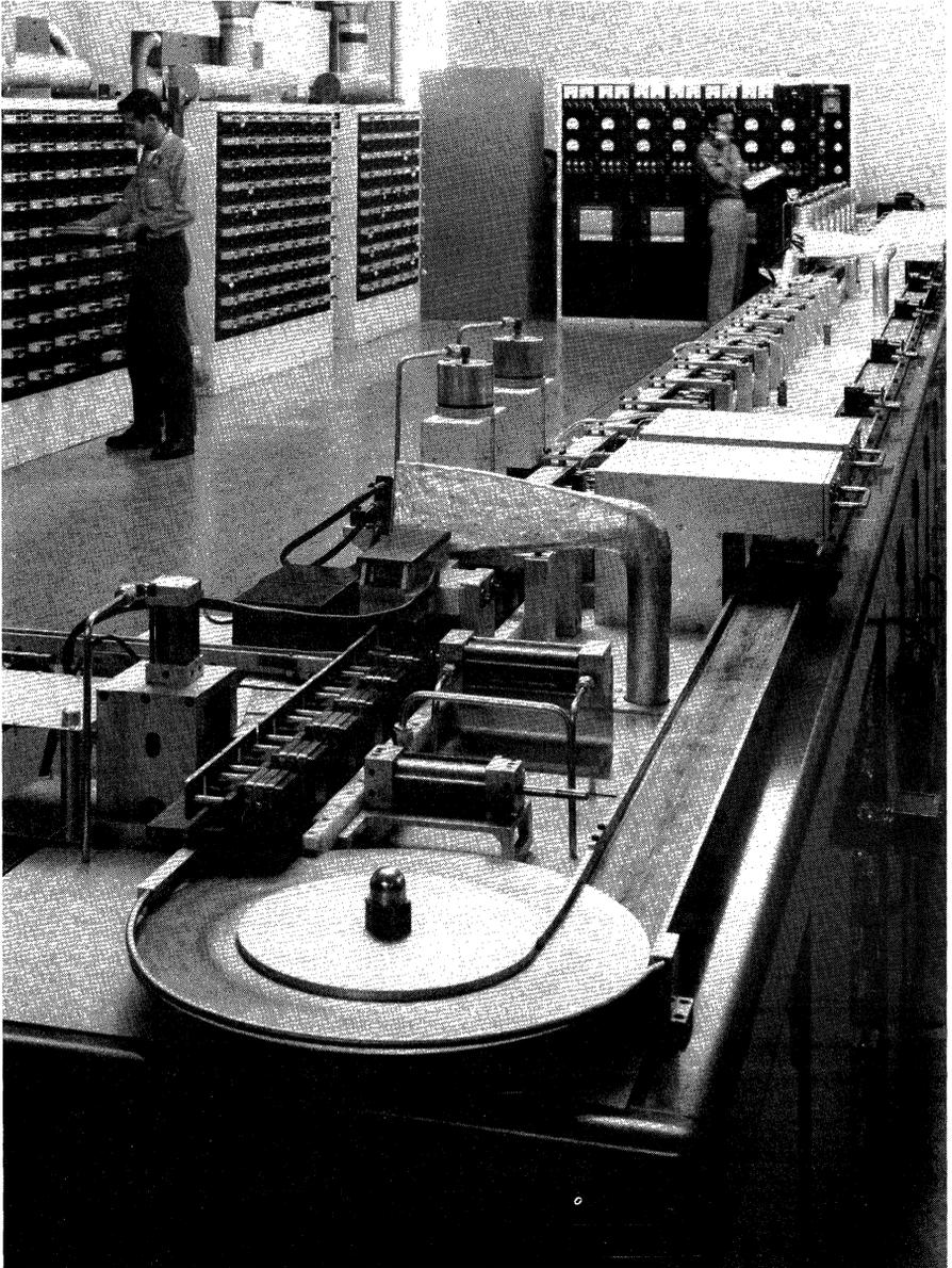
**This Central Automatic Recording and Testing facility (CART), designed and built by TI, automatically reads and records 10 parameters at two temperature levels on 1200 devices per hour.**
