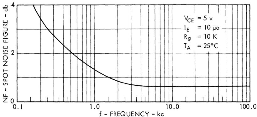
Fig. 2. Typical spot noise figure vs. frequency.
