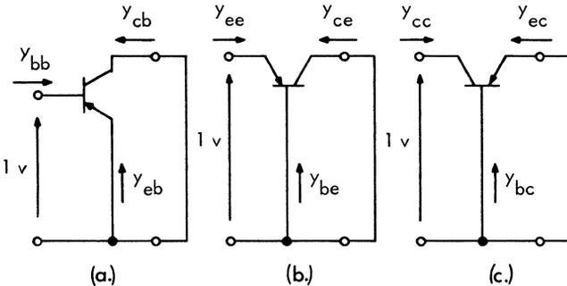
**Fig. 4. Orientations: (a) common emitter; (b) common base; (c) common collector.**
