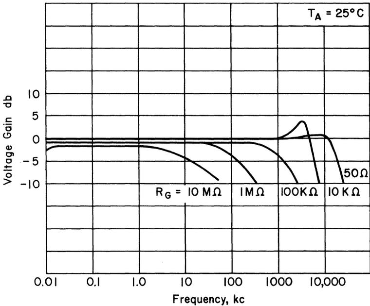
Fig. 37. Amplifier voltage gain vs. frequency.
