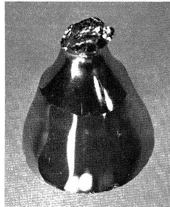
**Fig. 1.8.** Silicon crystal grown in  $[111]$  direction and showing pronounced  $(111)$  faceting.
