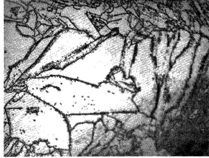
**Fig. 2.18.** Grain boundaries of a silicon boule delineated by selective deposition of SiO as the boule was held above the melt for a few minutes before cooling. Magnification approximately  $2\times$ .
