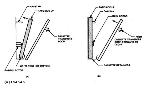
Figure 2-3. Tape Cassette Installation
