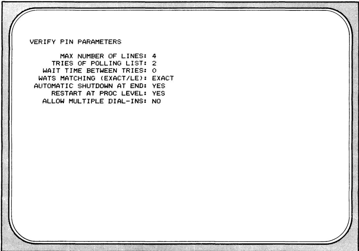
The response to MAX NUMBER OF LINES prompt is the number of lines to be supported by the Poller software on the user's system. The range of values is from 1 to 8; the default is 4. You need not change this value unless more than four lines are required.
