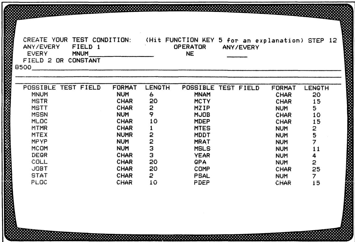
For the first prompt, enter ANY or EVERY. ANY means that only one occurrence in a record of FIELD 1 must meet the test condition for the condition to be true. EVERY means that every occurrence in a record of FIELD 1 must meet the condition for the condition to be true.
