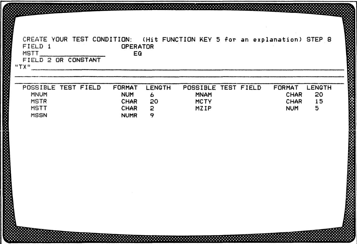
The first prompt requests the field ID or alias to be used as the first operand. The second prompt requests the relational operator for the condition: EQ for equal, LT for less than, and so on. The HELP screen for this step explains the relational operators.
