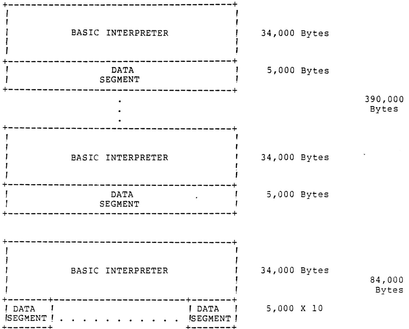
Figure 1-2 Saving Memory Through Segmentation
