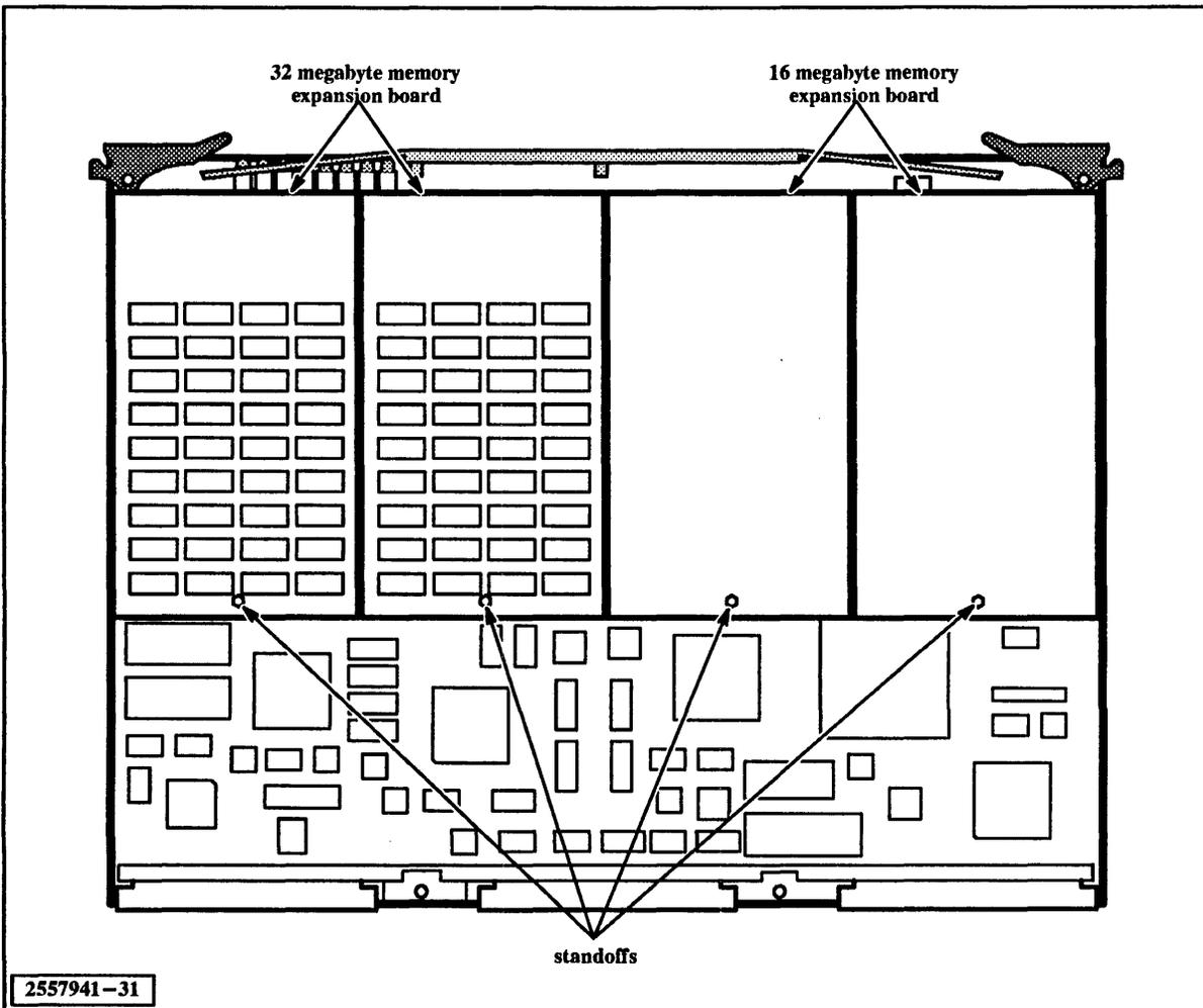
**Installing the Processor Board**
