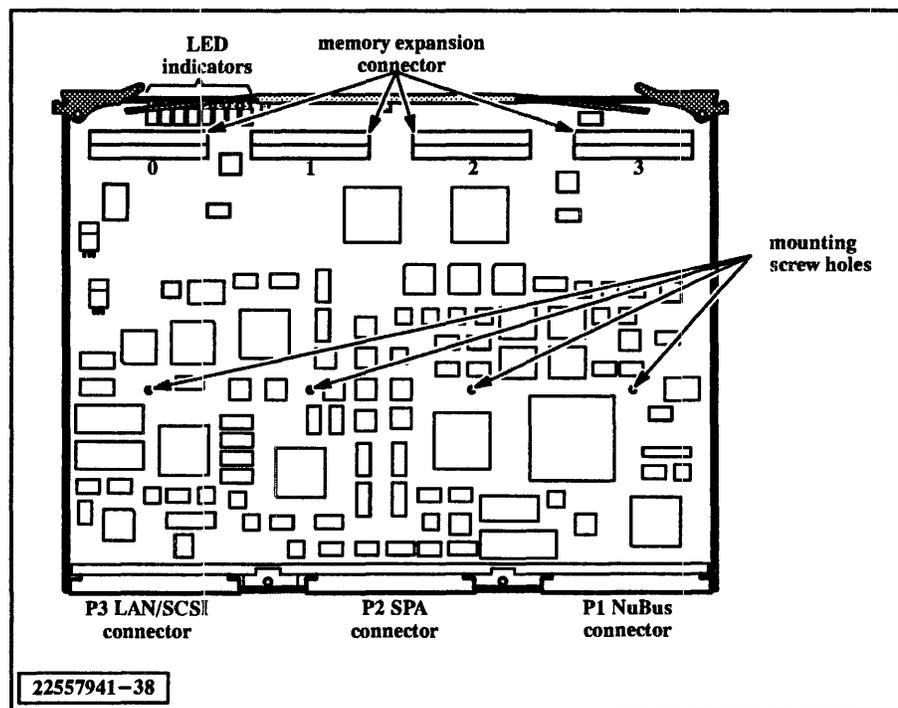
**Figure 3-3 Memory Expansion Mounted on the Processor Board**
