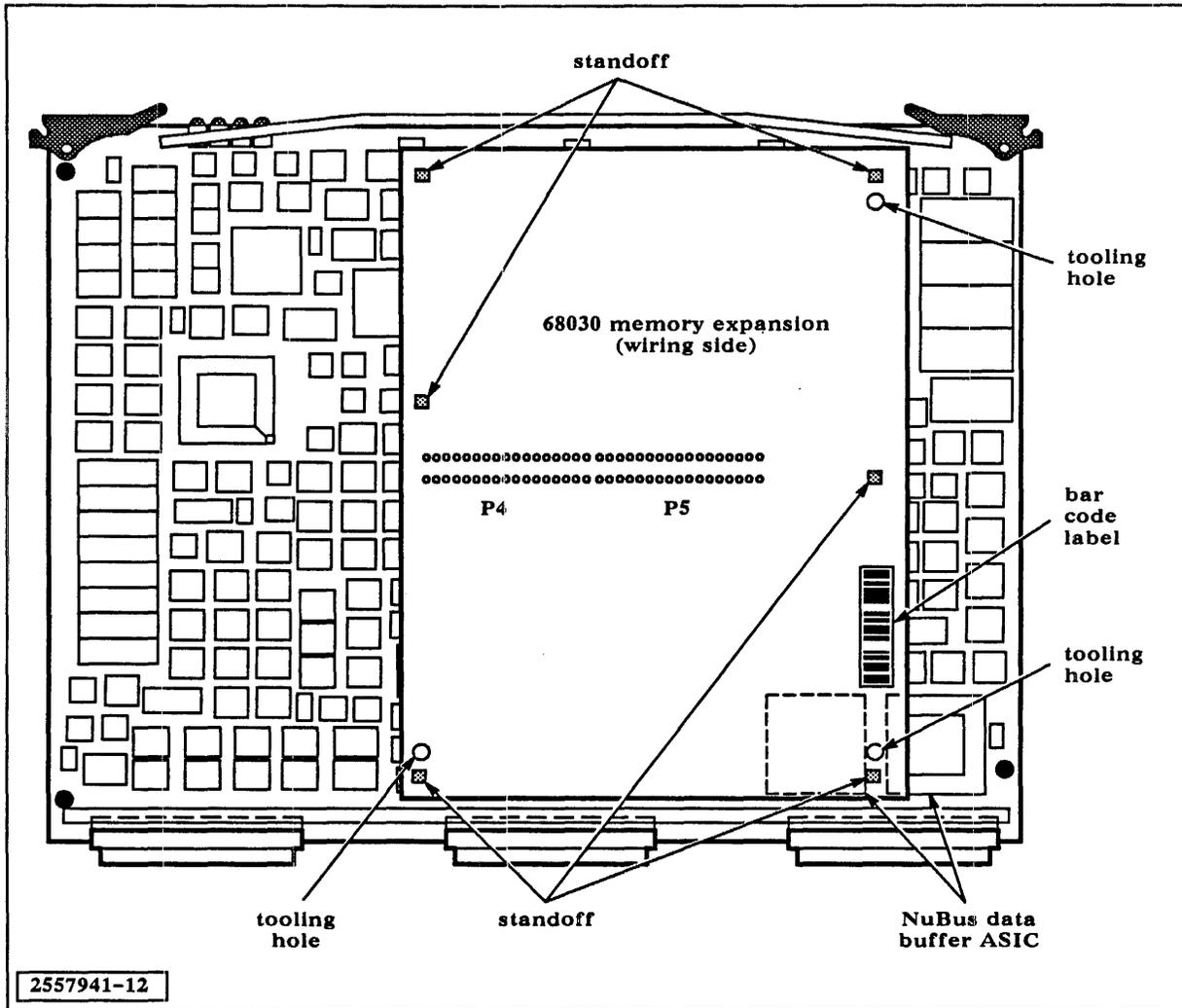
**Installing the Processor Board**
