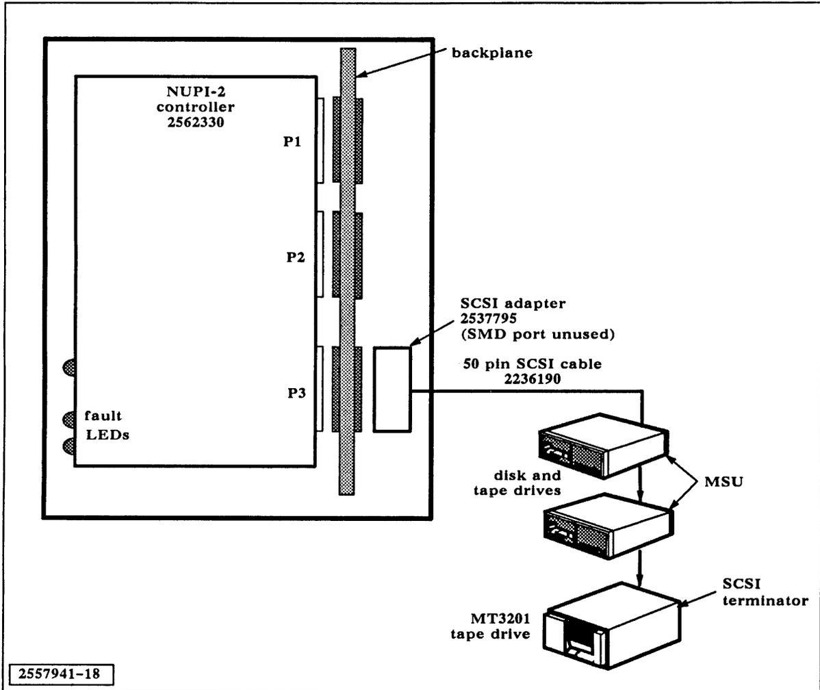
Figure 3-2 NUPI-2 Board Cabling to a PE-48
