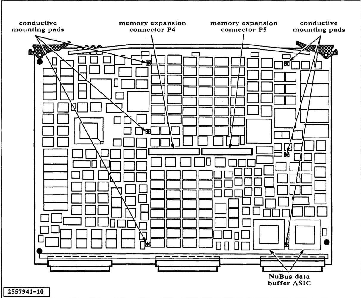
Figure 3-3 Memory Expansion Mounted on the Processor Board
