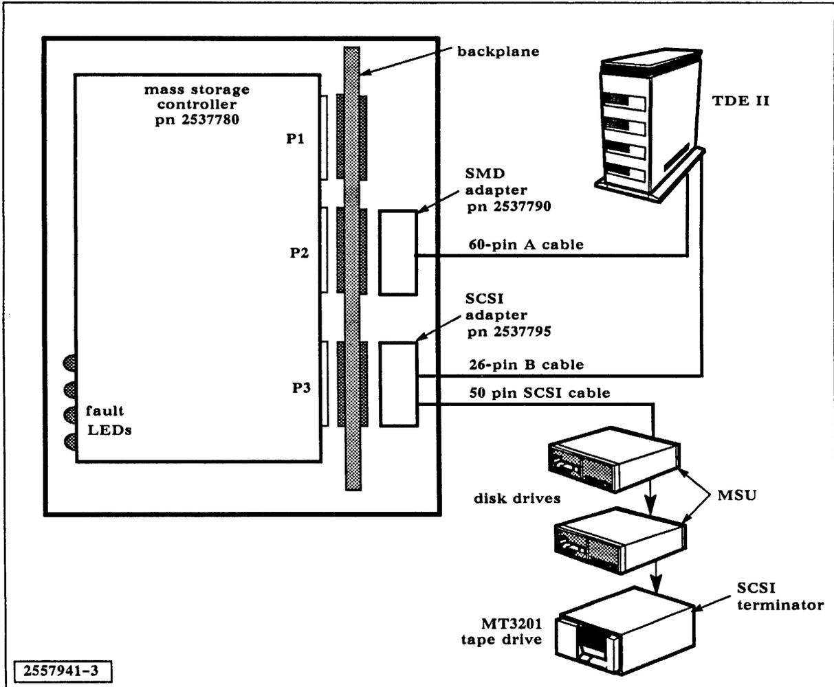
Figure 3-2 MSC Board Cabling to a PE-48
