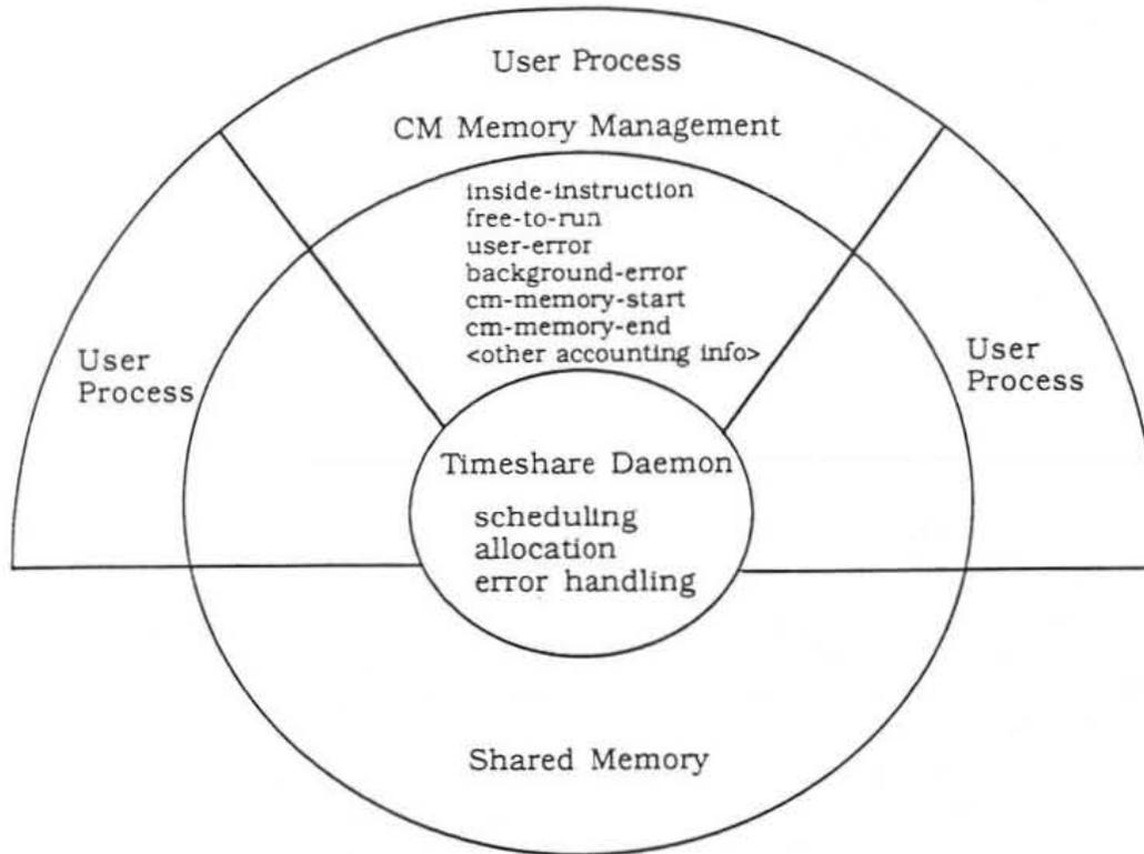
Figure 5: Timesharing control mechanism.
