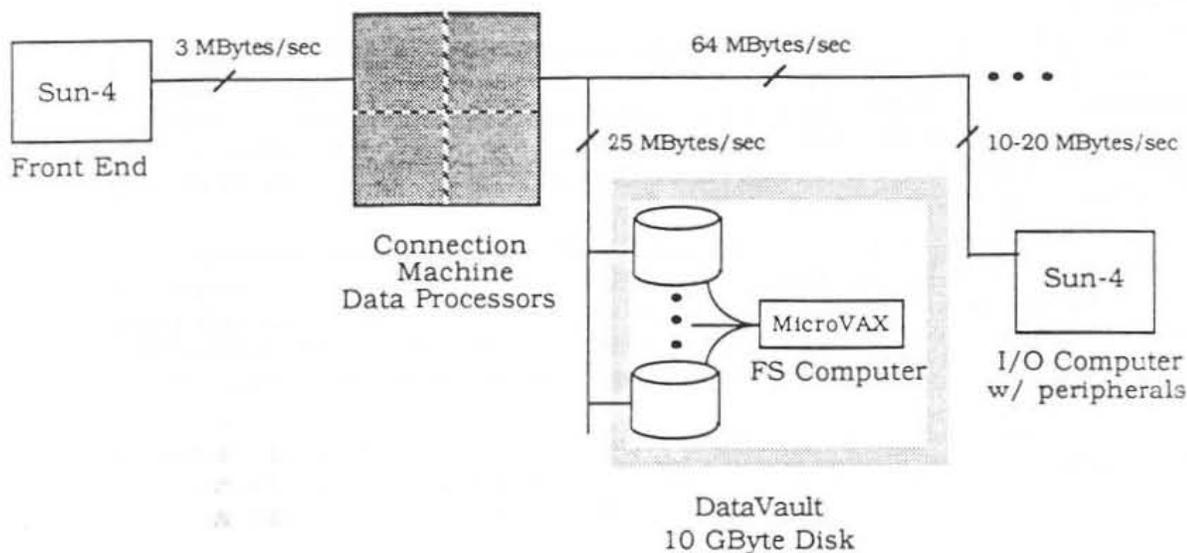
Figure 1: Example Connection Machine System
