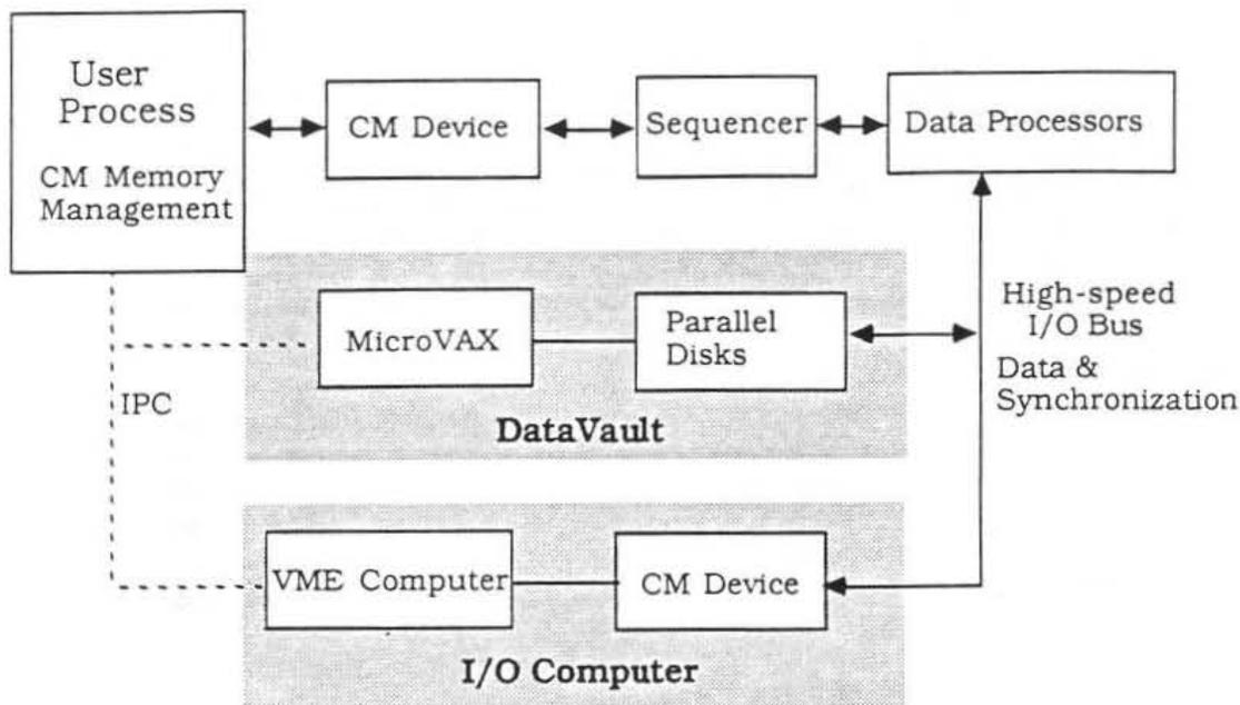
Figure 3: The front end and the I/O system.
