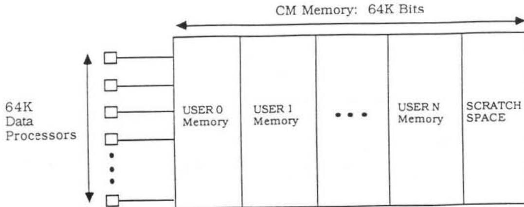
Figure 4: CM memory configuration under timesharing.
